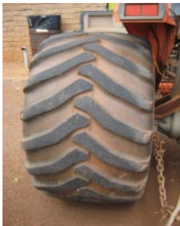
Mower tires are in need of replacement. Left tire has patches of rubber missing and right tire has worn tire tread.
