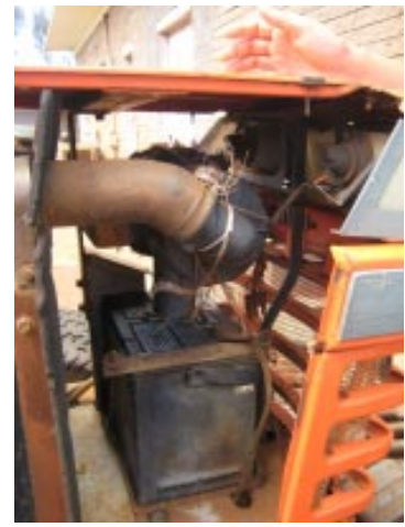
Side panels of mower were removed to prevent over-heating. Repairs to hold parts in place made use of rope.
