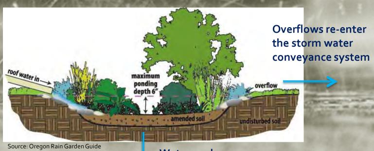
Soil microorganisms and plant roots break down pollutants.
