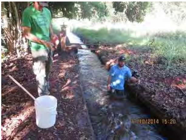
Measuring Ditch Flow Just Below Waiawa Hydropower Plant; Waiawa Reservoir
