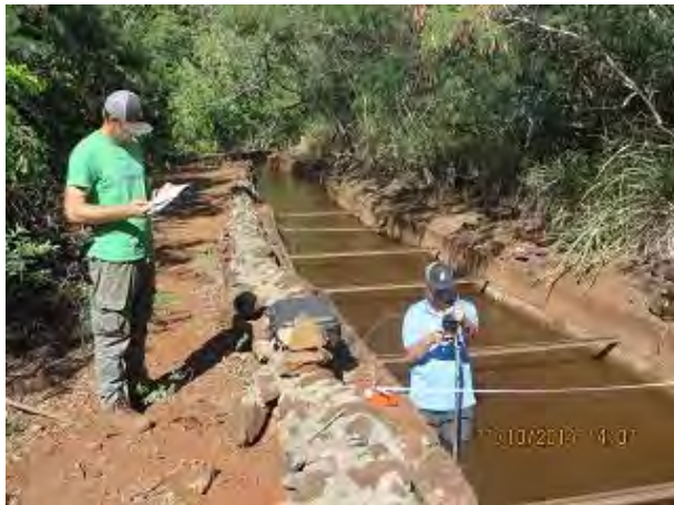
Measuring Ditch Flow Just Below Kōke'e Road Crossing; Ditch Leakage Just Above Road
