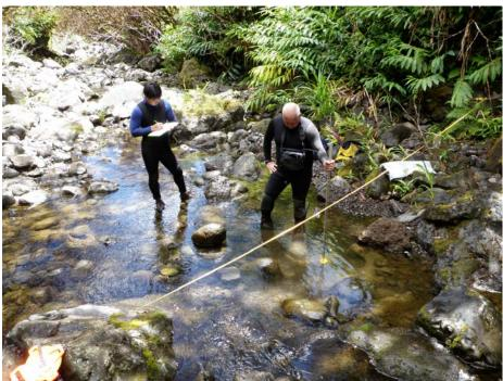
Figure 4-16. Stream flow measurements taken downstream of survey site 6 and below Hāna Hwy. (6/28/2009; Tributary name: (64023001); PBN: ts006p-003-062809; Surveyor: Shimoda, T.; Habitat type: Run; SBN: 123; Lat. (DD): 20.81002, Long. (DD): -156.09494).
