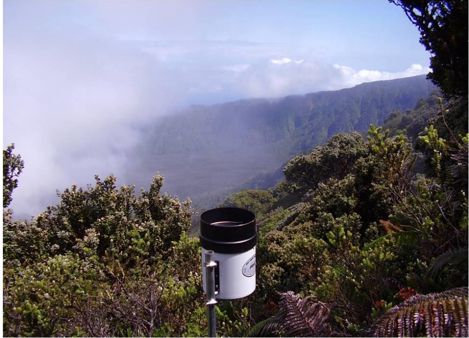
Rain gages provide much-needed monitoring of rainfall.
