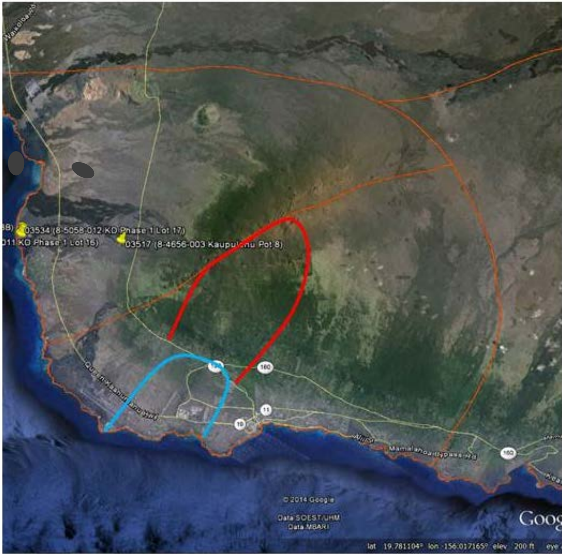
FOF Figure 11. Approximate areas in the high-level and brackish basal aquifers that contribute ground water flow to the shoreline between Honokohau Harbor and Keahole Point.
