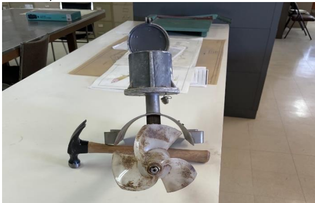
1) Front-view of the propeller flow meter used by WWC.
