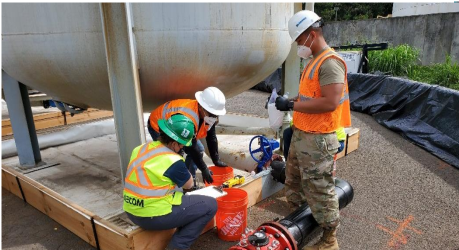
Sampling of 5MGD GAC Effluent
