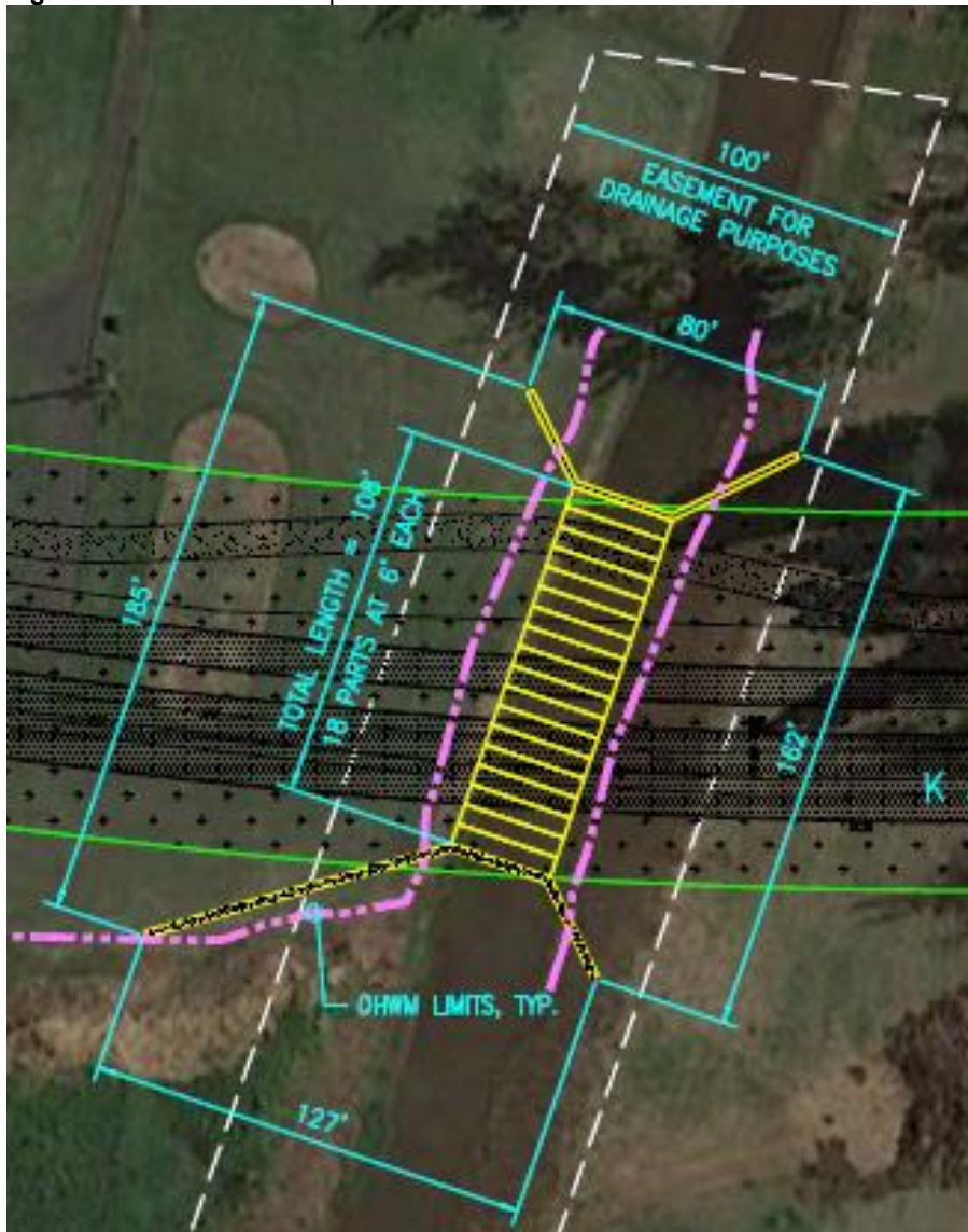
Figure 2: Plan view of Conspan culvert installation.
