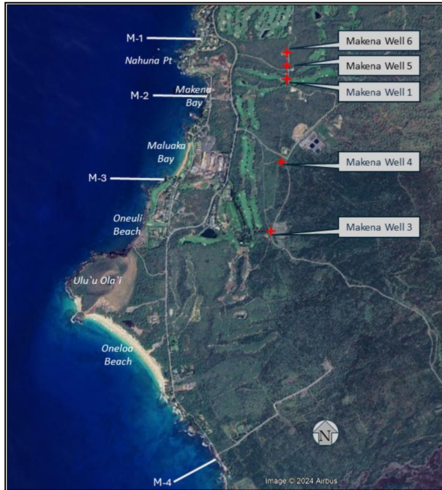
Figure 2. Location of water quality monitoring transects (M-1 through M-4) and resort irrigation wells.
