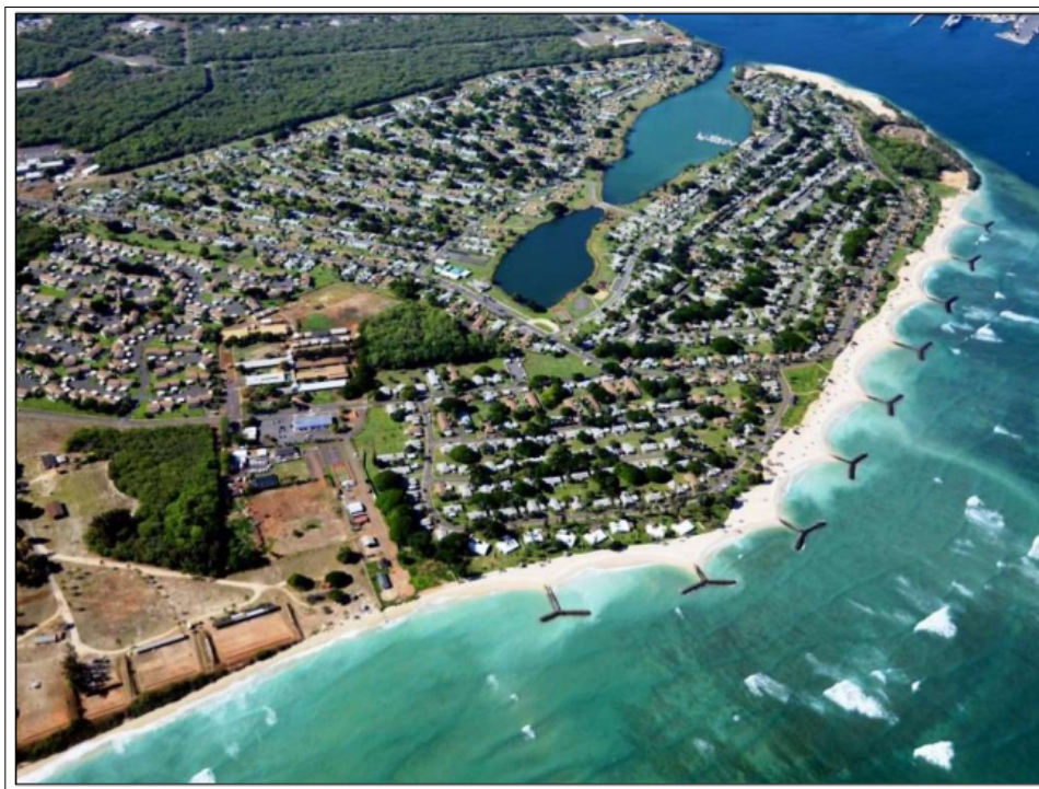
Example of Beach Nourishment with T-Head Groins (Iroquois Point, O'ahu, Hawai'i)
