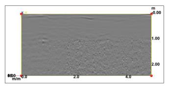
Figure 61. GPR Grid 3 reflection profile at 6.0 m from the grid origin showing signal attenuation at approximately 1.0 m below surface indicative of the presence of water saturation or the water table
