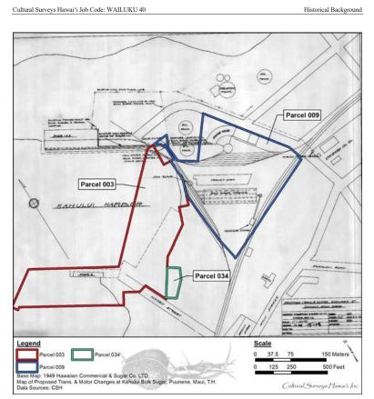
Figure 52. 1949 HC&S map showing then proposed changes to the transportation and infrastructure for the bulk sugar plant; note CSH 2 in center, and CSH 4 extending along the wharf (HC&S 1949)
