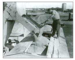
Figure 33. Bulk sugar being loaded into transport trucks to be carried to the bulk sugar plant storehouses, circa 1940s; conveyor system (CSH4) visible in background (photo courtesy of HC&S Sugar Museum)
