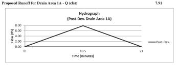
Prop. Runoff Volume (area under hydrograph) =  $Q_{peak} \times T_{conc} \times 60$  seconds/minute =
