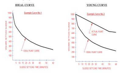
When the curve tends to rise from the ideal plant curve, as depicted in Example Curve No.2 (usually accompanied by excessive white sudsy foam in the aeration basin), the sludge age is probably young and the return sludge rate from the clarifier should be adjusted. This is usually done in steps of 20 percent increase at one time. This also should be accomplished by decreasing the sludge wasting from the system and reducing the air into the aeration basin.
