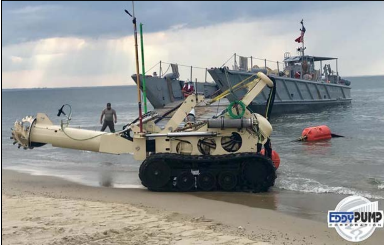
Figure 3-10 Remote Operated Submersible Dredge (Eddy Pump®, 2021)
