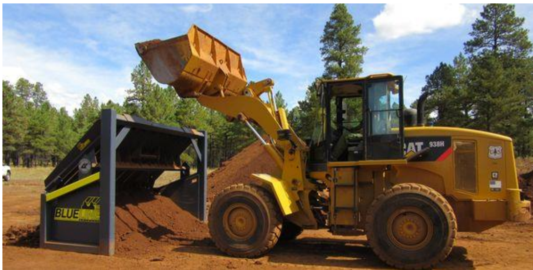
Figure 5-30 Grizzly rock screen used to separate coarse material
