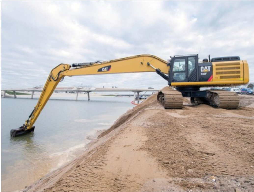
Figure 7-20 CAT 352F LRE long reach excavator ( www.caterpillar.com )
