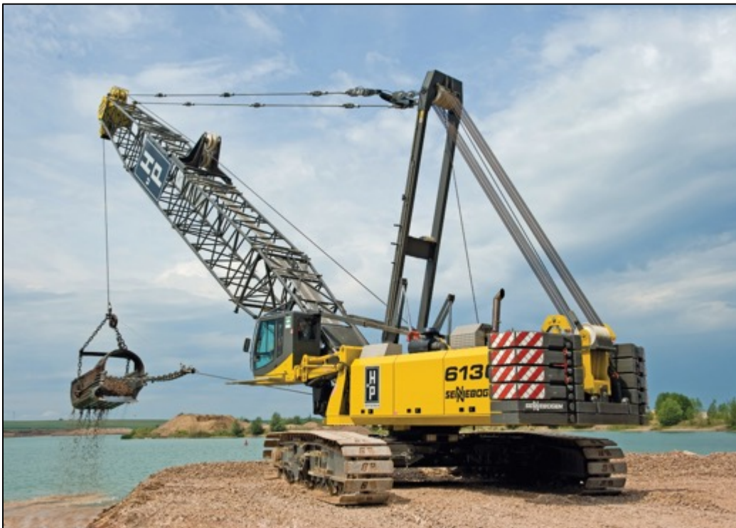
Figure 7-21 Sennebogen 6130 HD duty cycle crawler crane ( www.sennebogen.com )
