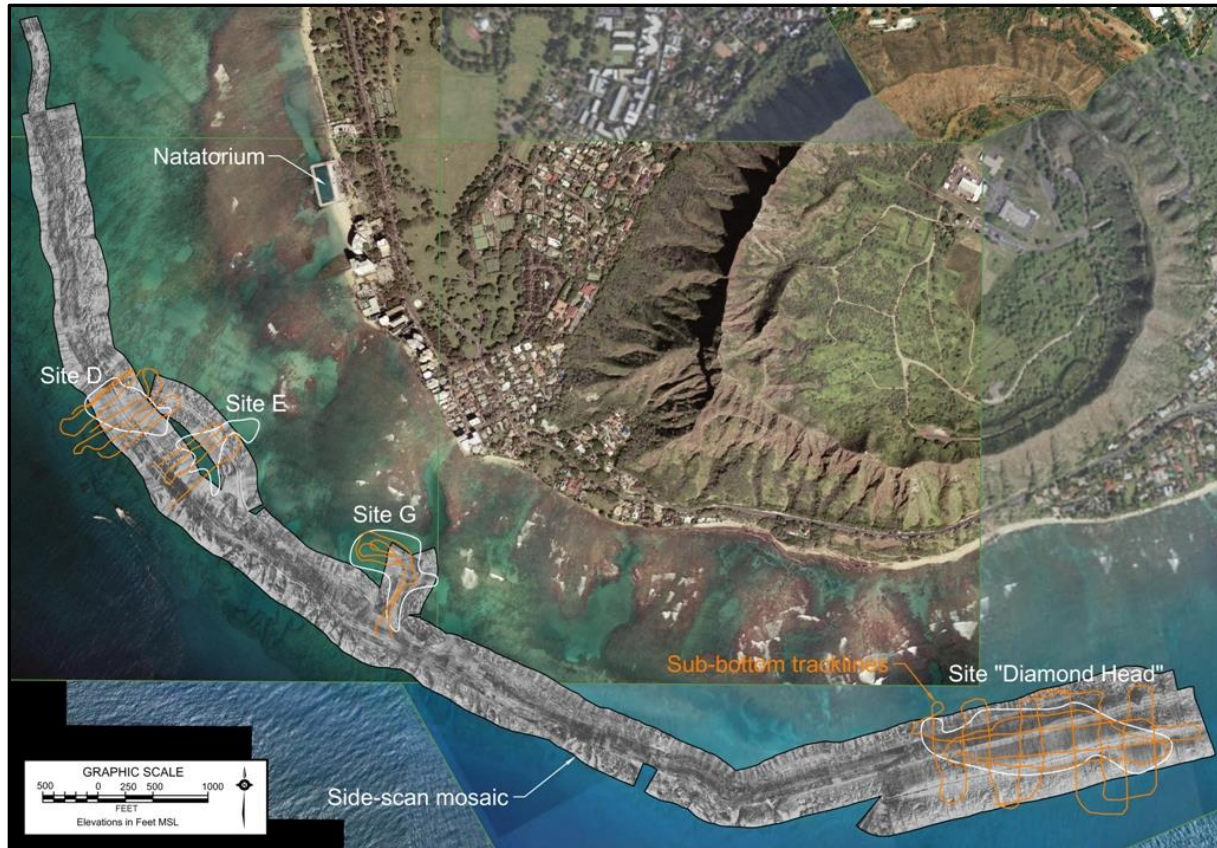
Figure 3-11 Side-scan sonar mosaic and sub-bottom profiler tracklines
