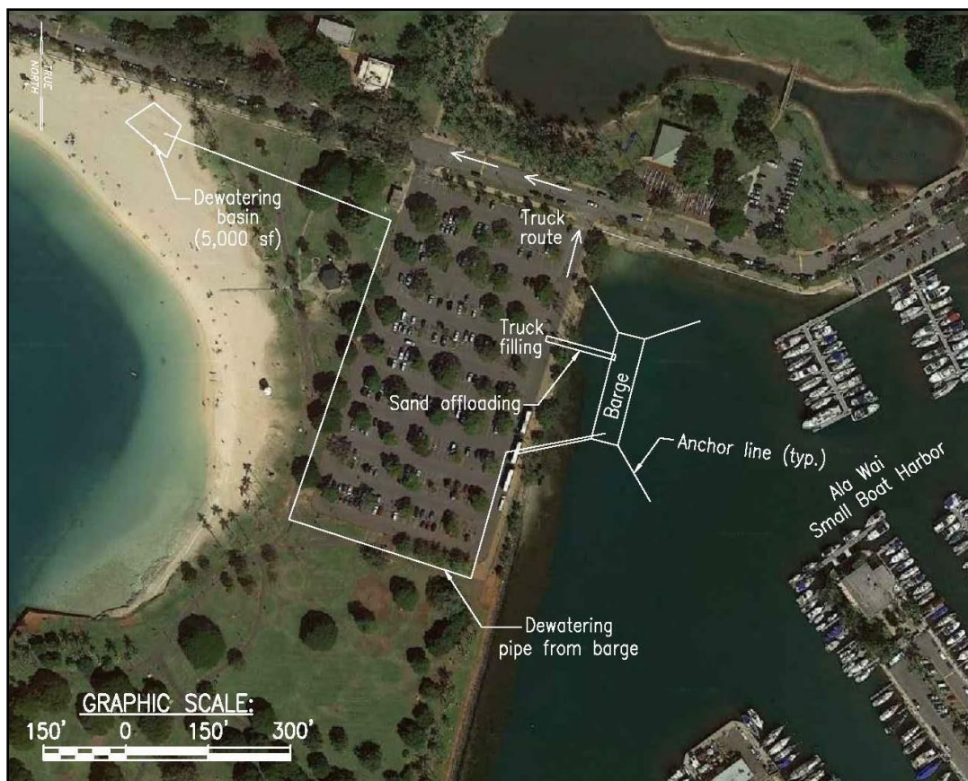
Figure 5-13 Example of barge offloading at Ala Wai and Magic Island
