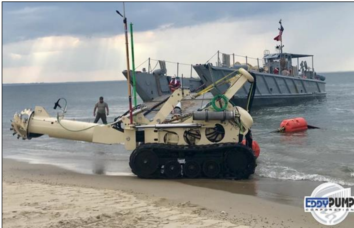
Figure 5-9 Remote Operated Submersible Dredge (Eddy Pump, 2021)
