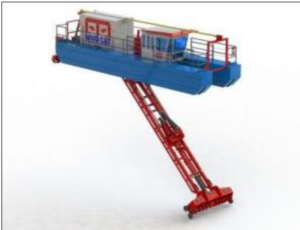
Figure 5-8 Example of hydraulic suction dredge (Ellicott Dredges)
