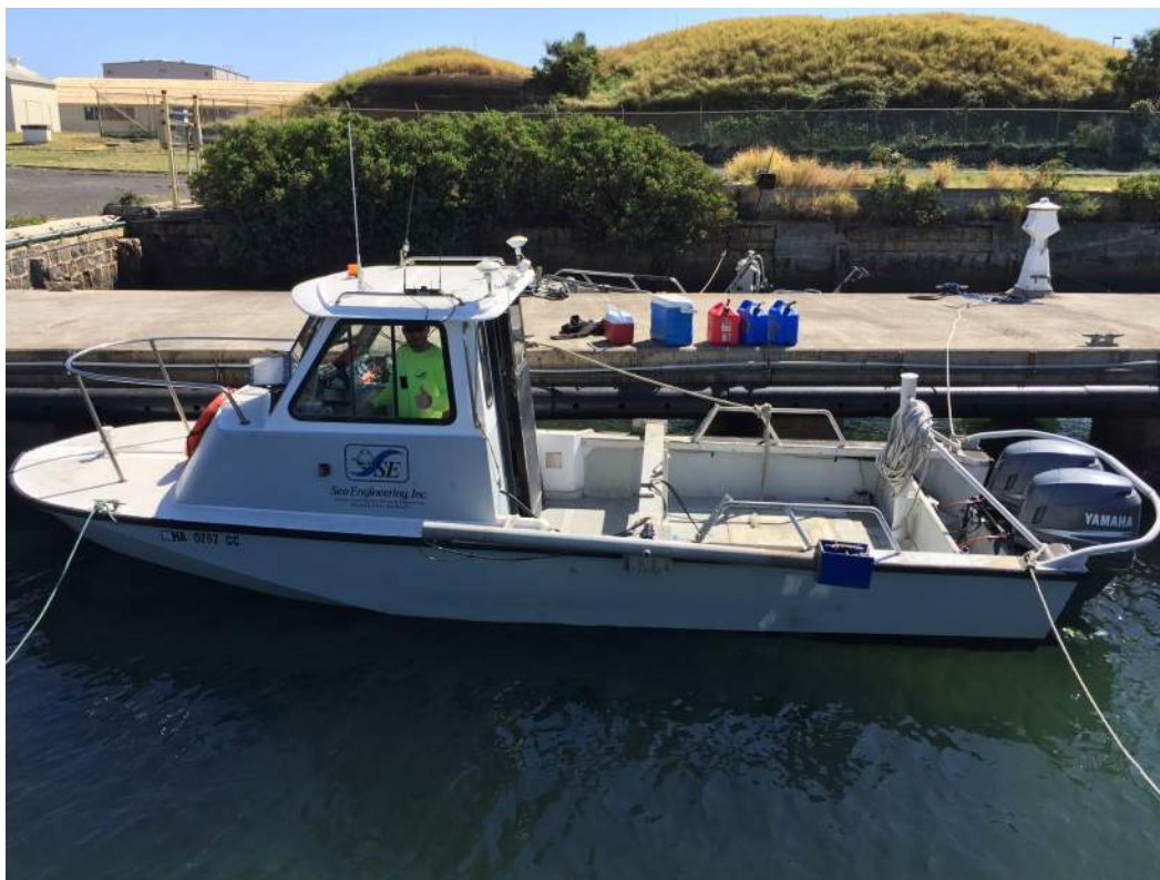
Figure 3-1. SEI's survey boat 25-ft Whaler – multibeam mount at center front, rotated up
