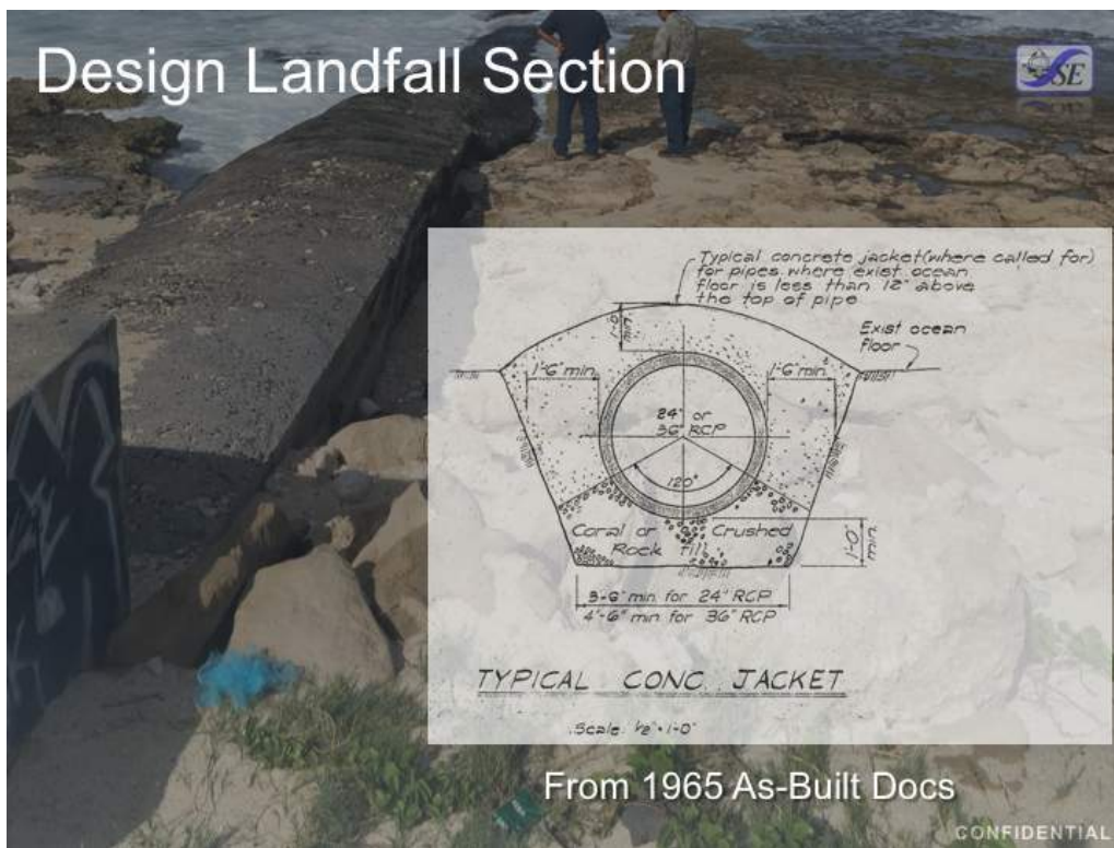
Figure 5-3. Outfall landing typical design cross section
