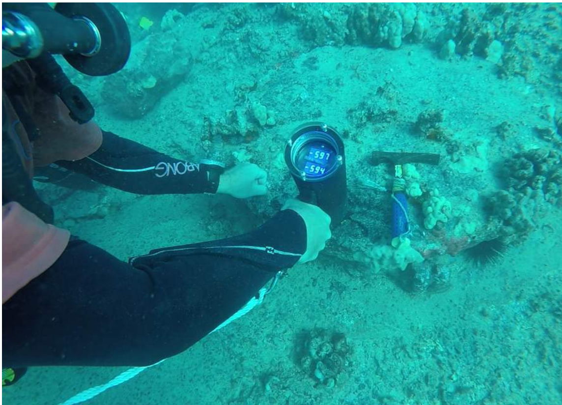
Figure 4-25. Inspector shown obtaining galvanic potential measurements with CP-gun at MH 4.
