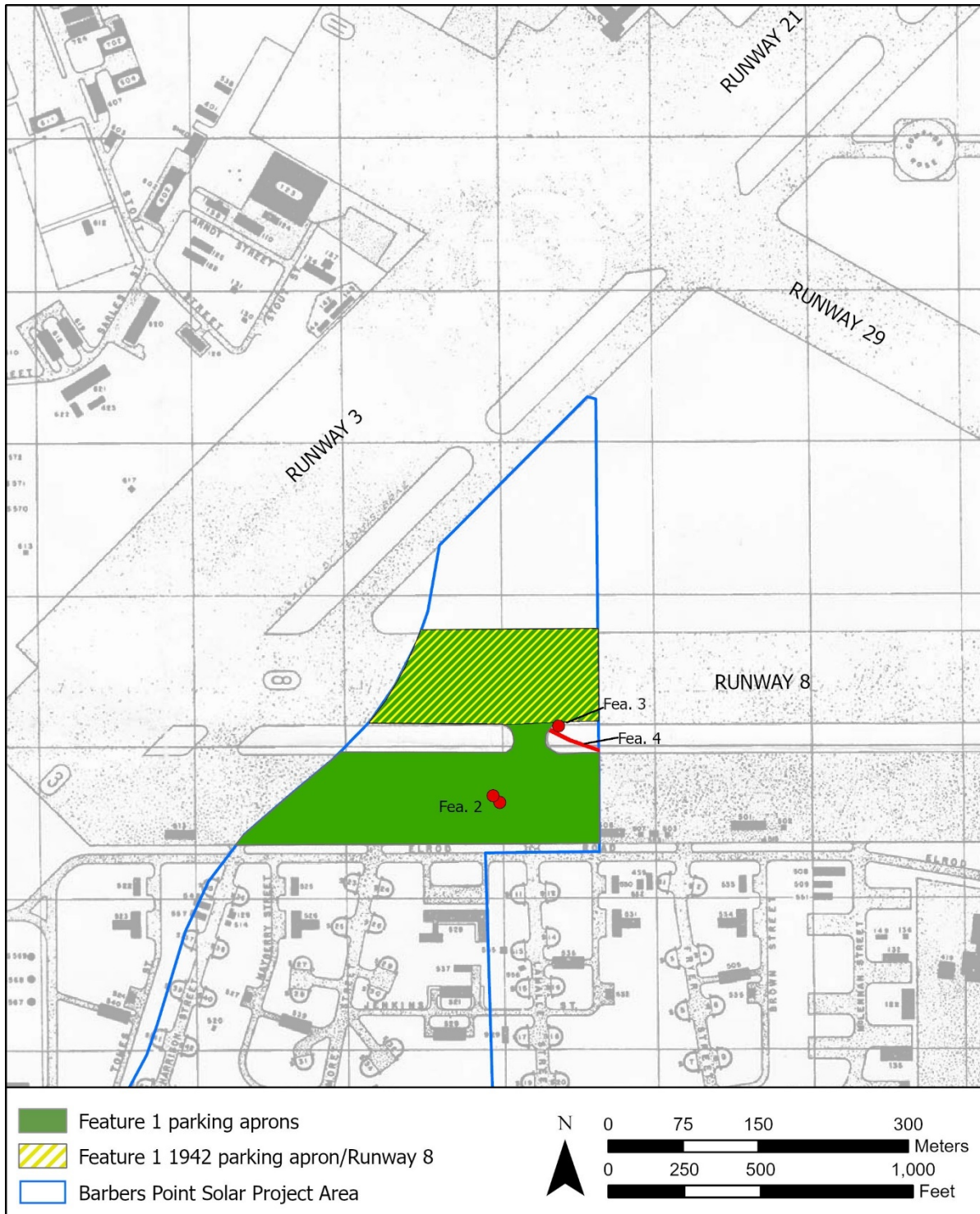
Figure 248. Plan-view map of Site T-08 WWII runway infrastructure overlaid on MCAS Ewa map (U.S. Navy 1948).
