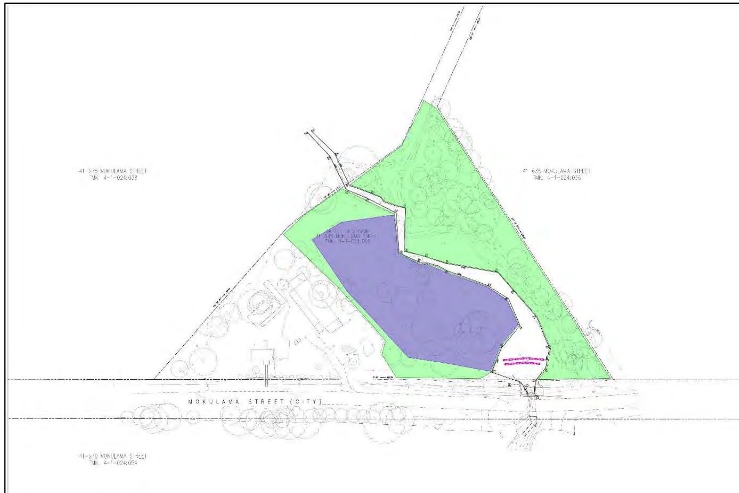
Figure 4. Project map (supplied by Okahara and Associates, Inc. 2022) with north to the right and Mokulama Street, which is to the east, at bottom. Grading will be required in the area highlighted purple within the interior of the reservoir which will then be grassed and maintained. Vegetation, including all trees within the property, will be cleared within the area highlighted green. Two rows of staggered bollards intended to capture debris are proposed and depicted with the magenta lines near the reservoir spillway (close to Mokulama Street).
