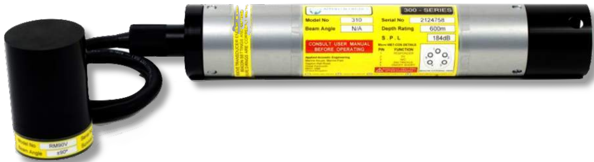
Figure 4-6. Applied Acoustics' Easytrak Nexus Lite™ USBL transponder model used at Waianae
