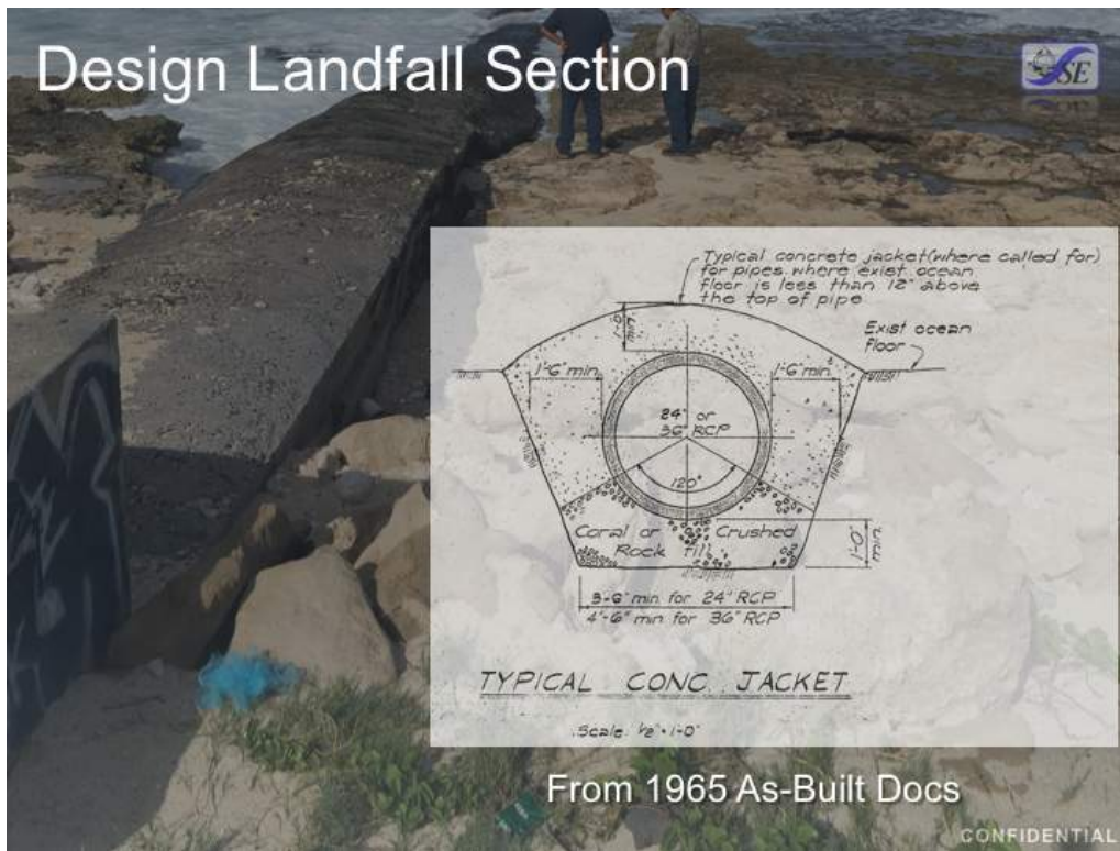
Figure 5-3. Outfall landing typical design cross section
