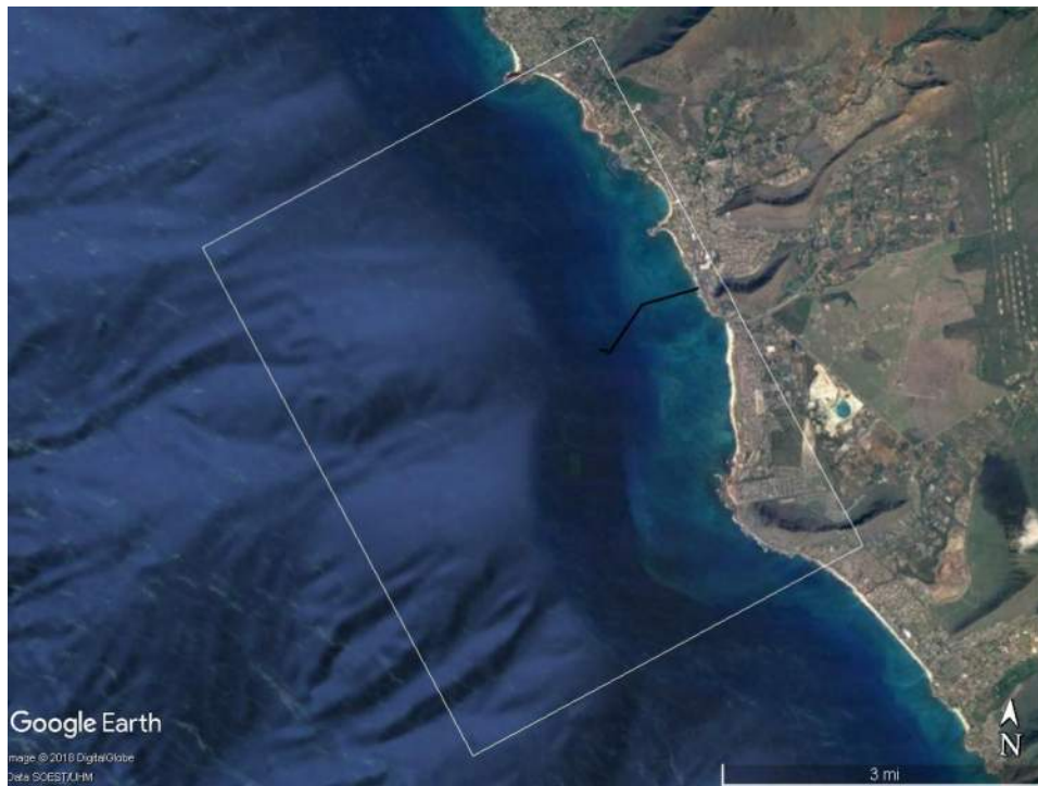
Figure 6-30. Boundaries of the Delft3D-WAVE/FLOW domain relative to the outfall.
