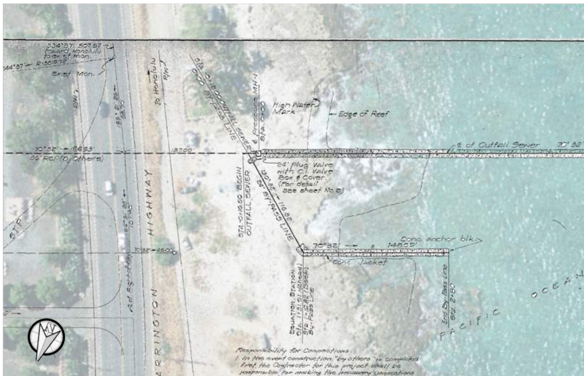
Figure 5-8. Outfall landing condition, 2007, with as-built plan overlay (source: UH CGG, 2019)
