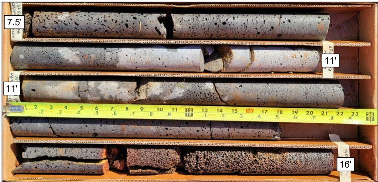
Boring B4 from 7.5 to 16 feet
