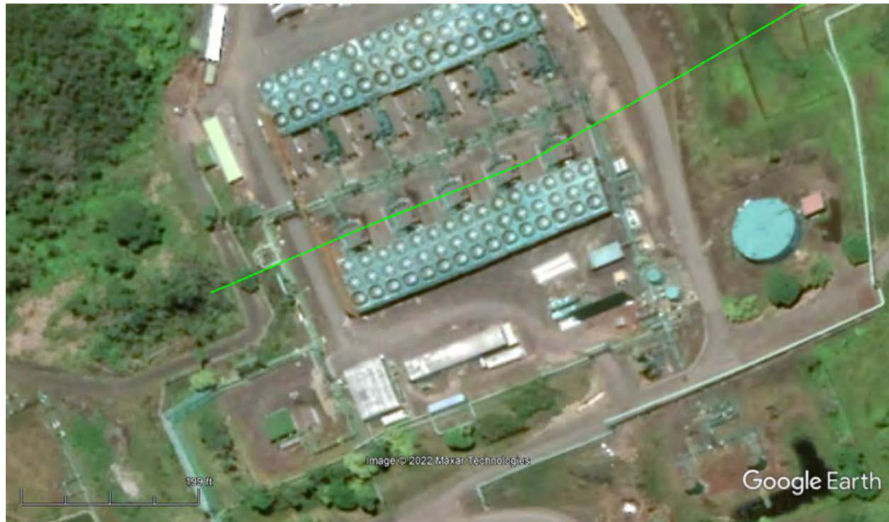
Figure 9 - PGV located directly over 1955 fissure line
