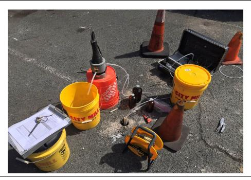
Groundwater purging and sampling of temporary wells were performed using a low-flow sampling technique.
