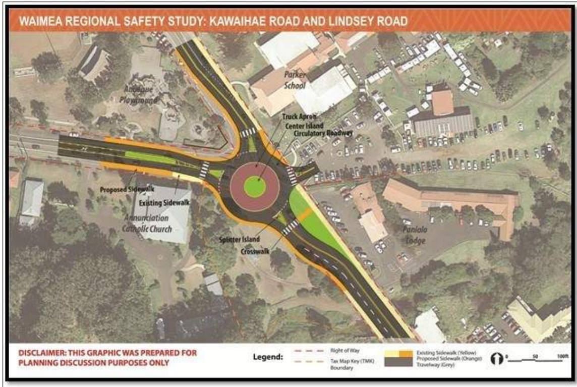
Figure 4. Kawaihae Road and Lindsey Road roundabout conceptual plan.
