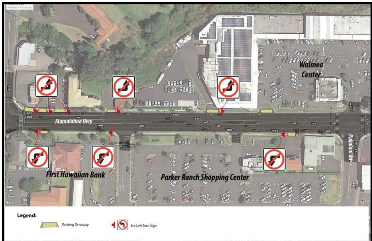
Figure 5. Conceptual Plan for Improvements to Mamalahoa Highway Between Lindsey Road and Pukalani Road
