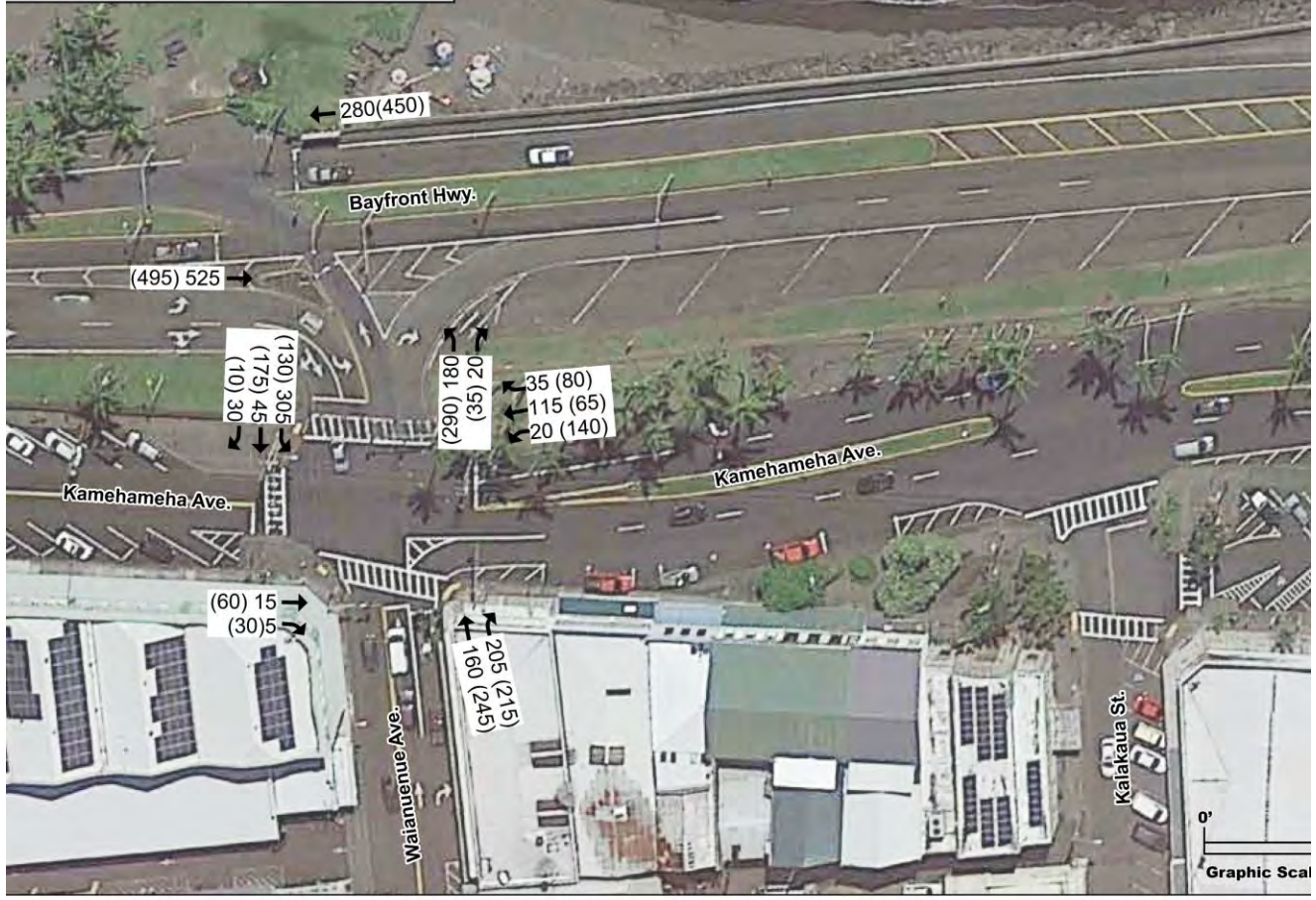
FUTURE YEAR 2025 VEHICLE PEAK HOUR SUMMARY Hilo Bayfront Highway Intersection Improvements Alternative Analysis
