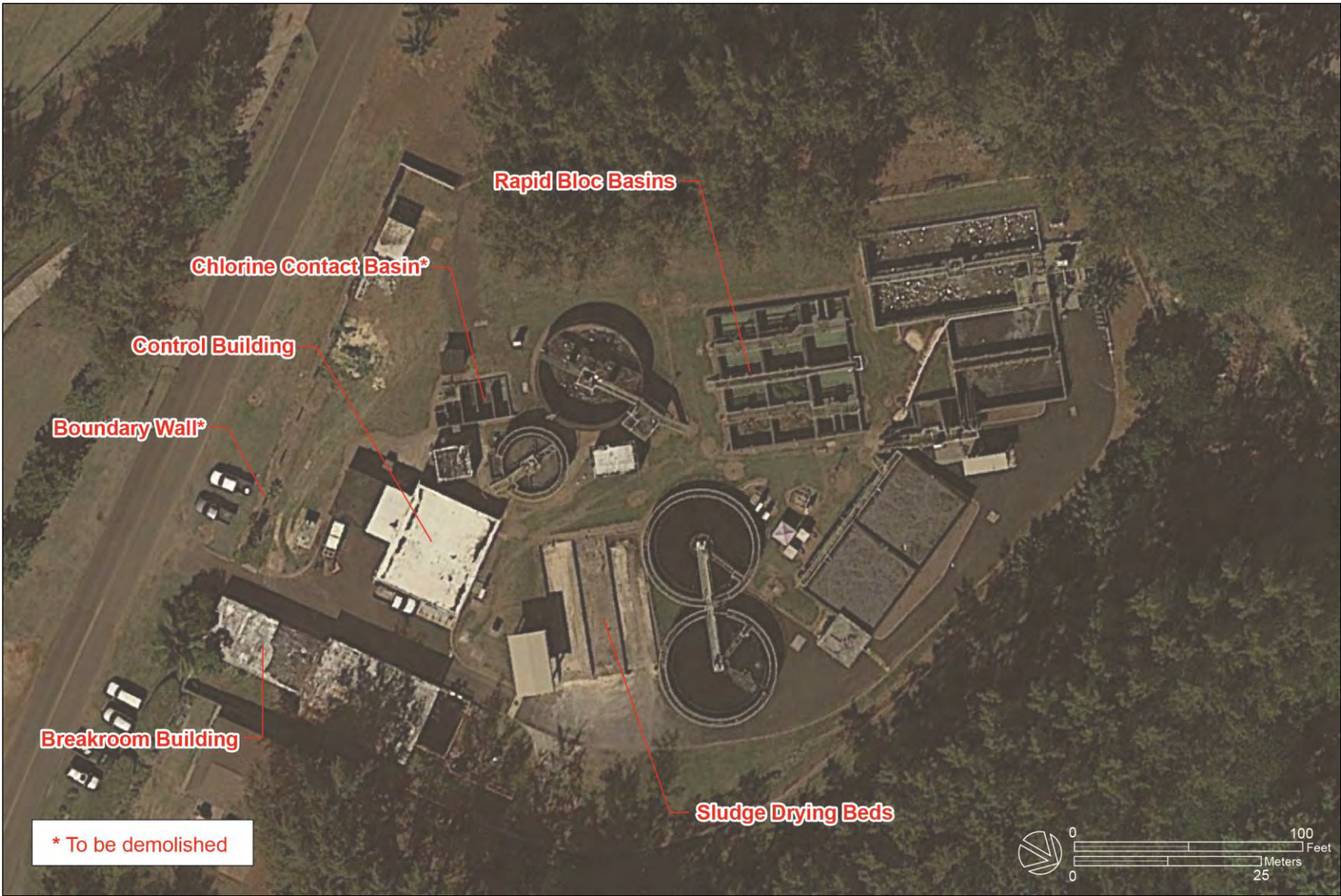
Figure 14. Wailua Wastewater Treatment Plant, Current Site Layout.
