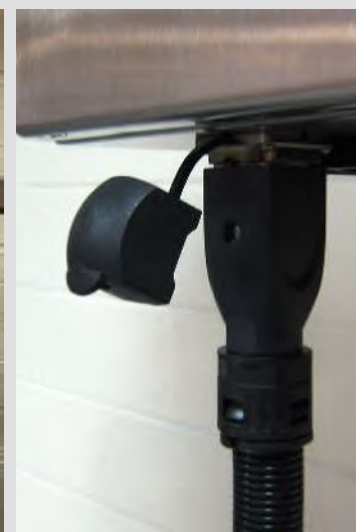
Modules connect to BCC via IP65 waterproof connectors
