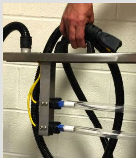
Modules connect to BCC via IP65 waterproof connectors
