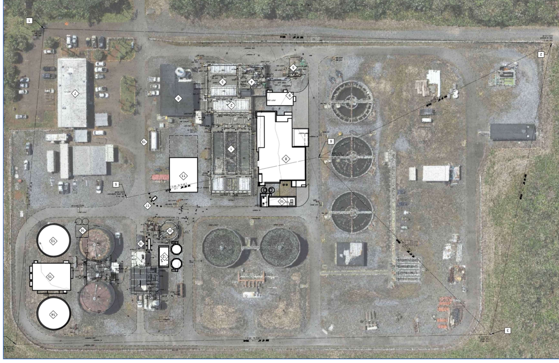
Figure 2 – Hilo WWTP aerial view showing locations of proposed new buildings and structures in white.
