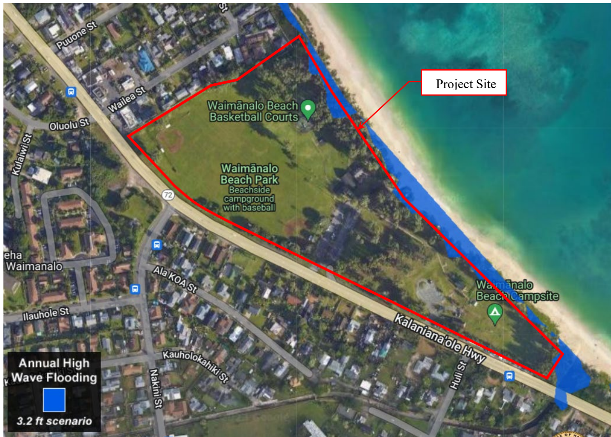
Figure 3-7: Annual High Wave Flooding in Project Area under a 3.2-foot Sea Level Rise Scenario
