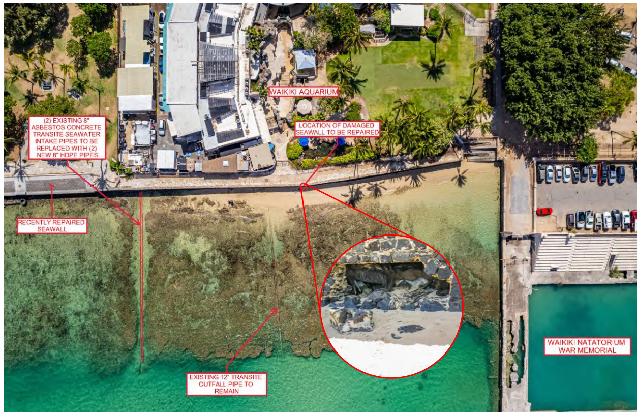
Figure 3-6: Location of Damaged Seawall to be Repaired
