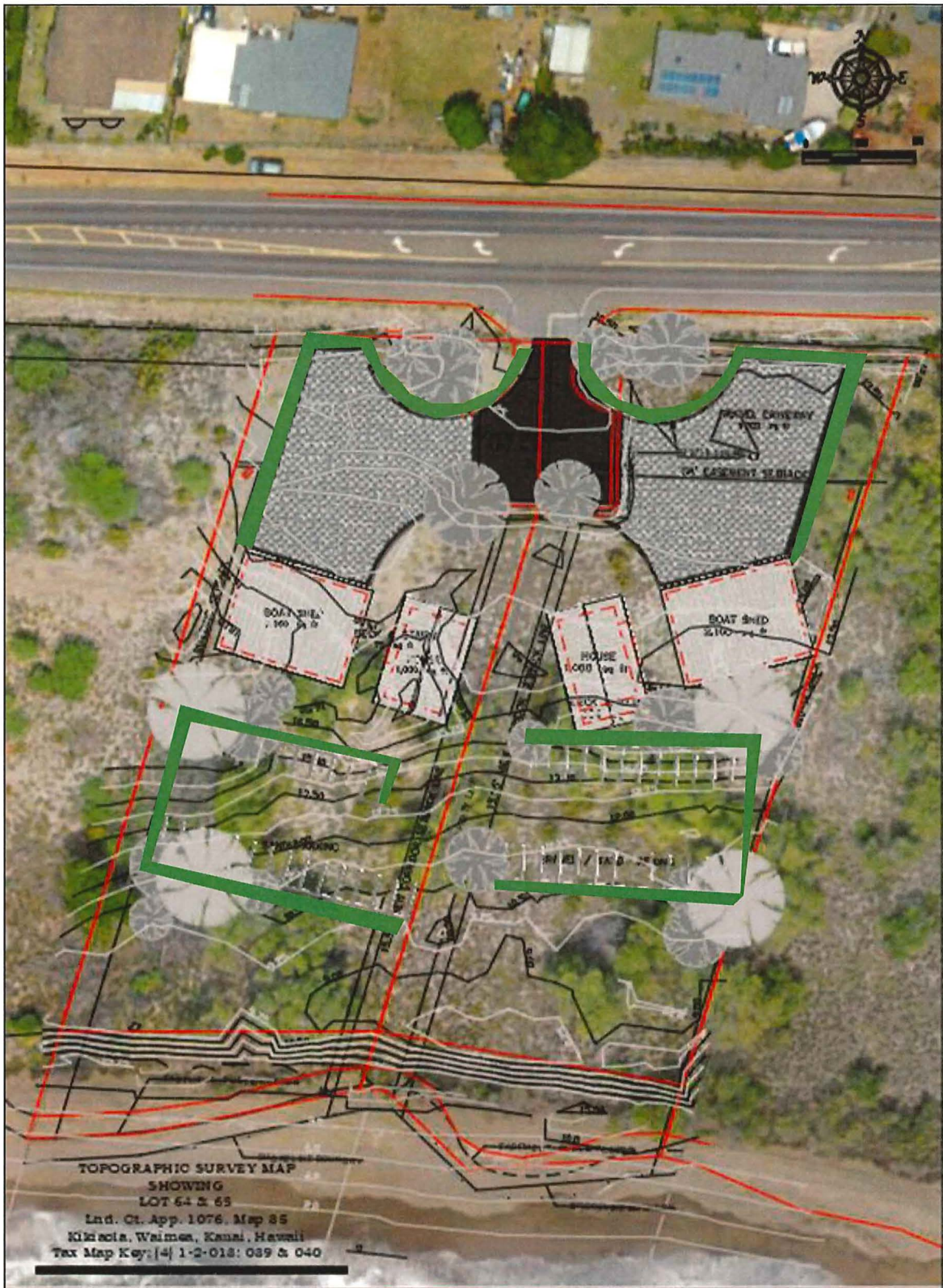
Figure 5-14: Example of vegetated swales located around paved areas.
