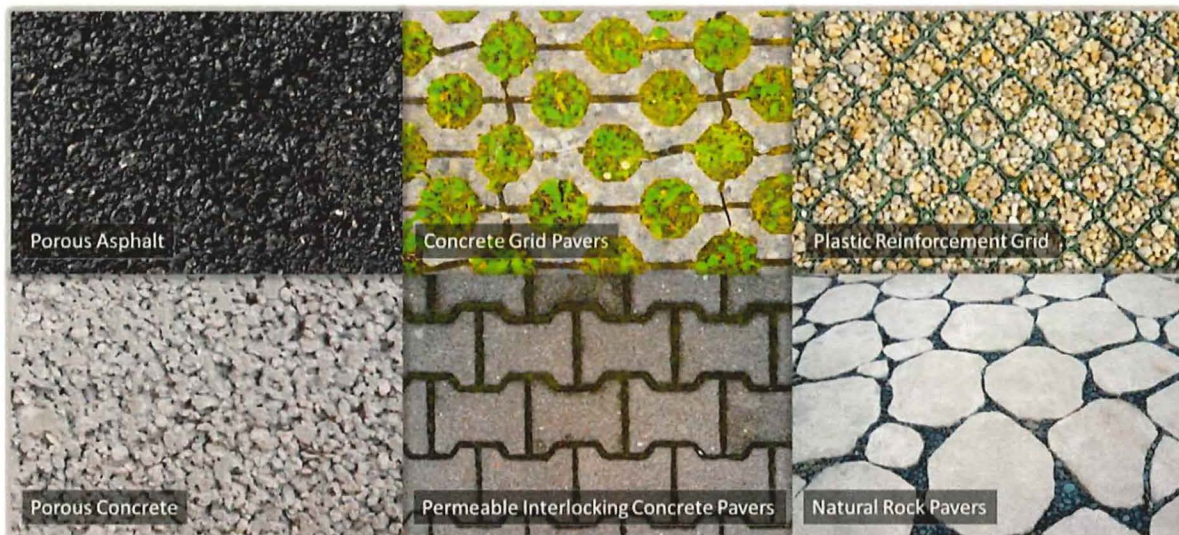
Figure 5-13 Some examples of pervious pavement types (Sprouse, 2020).
