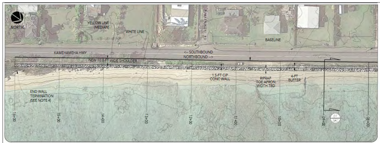
Figure 2-4. Plan view concept drawing of a proposed hybrid seawall with armor stone apron.
