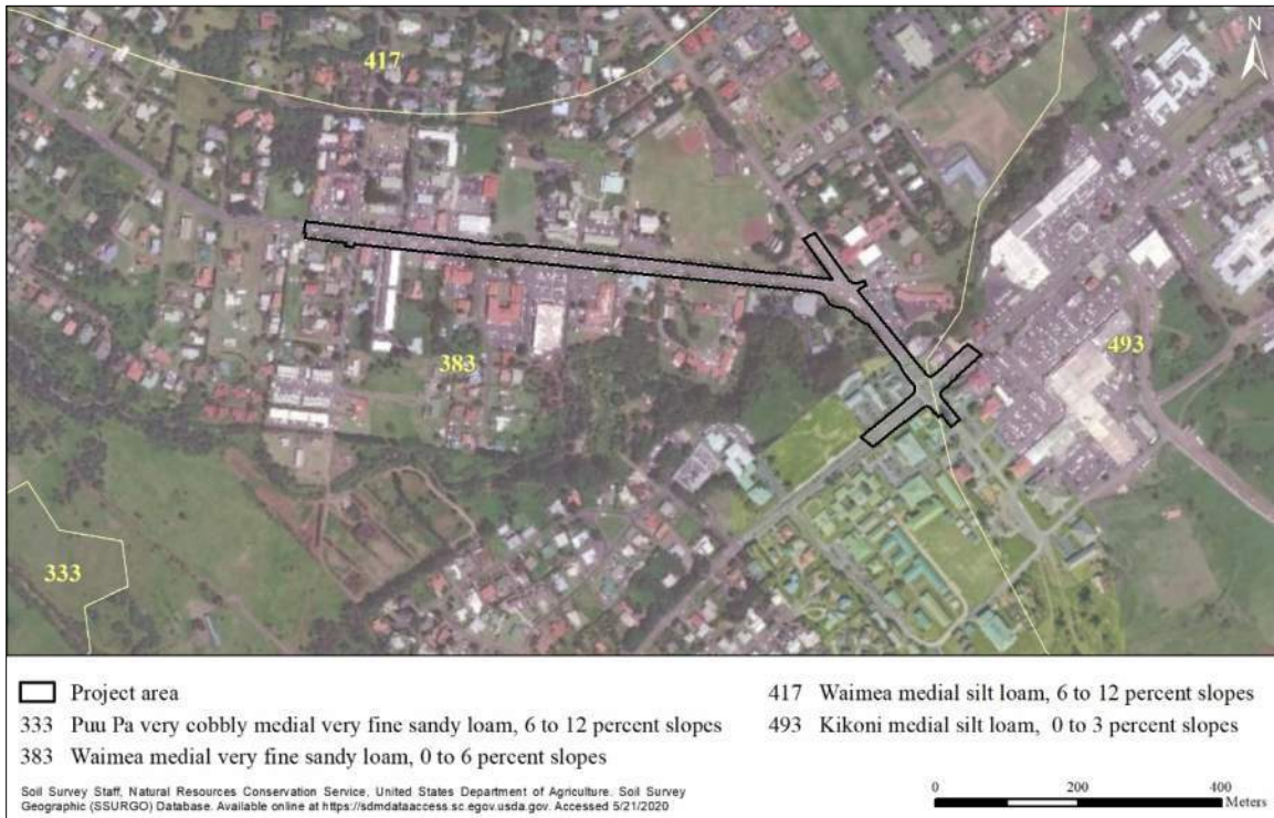
Figure 8. Soils in the project area.
