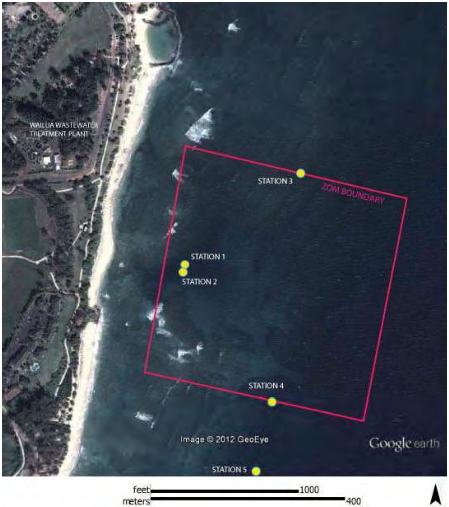
FIGURE 1. Aerial photograph of ocean off of Wailua Wastewater Treatment Plant on eastern shoreline of the Island of Kauai showing locations of five biological monitoring survey stations. Stations 1 and 2 are located adjacent to the ocean outfall diffusers; Stations 3 and 4 are located on the northern and southern boundaries of the Zone of Mixing, and Station 5 is a control station south of the Zone of Mixing.
