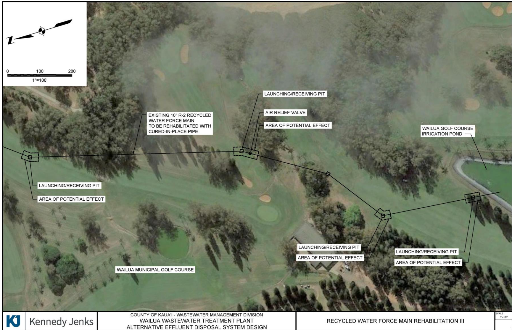
Figure 2-4: Recycled Water Force Main Rehabilitation at the Wailua Municipal Golf Course
