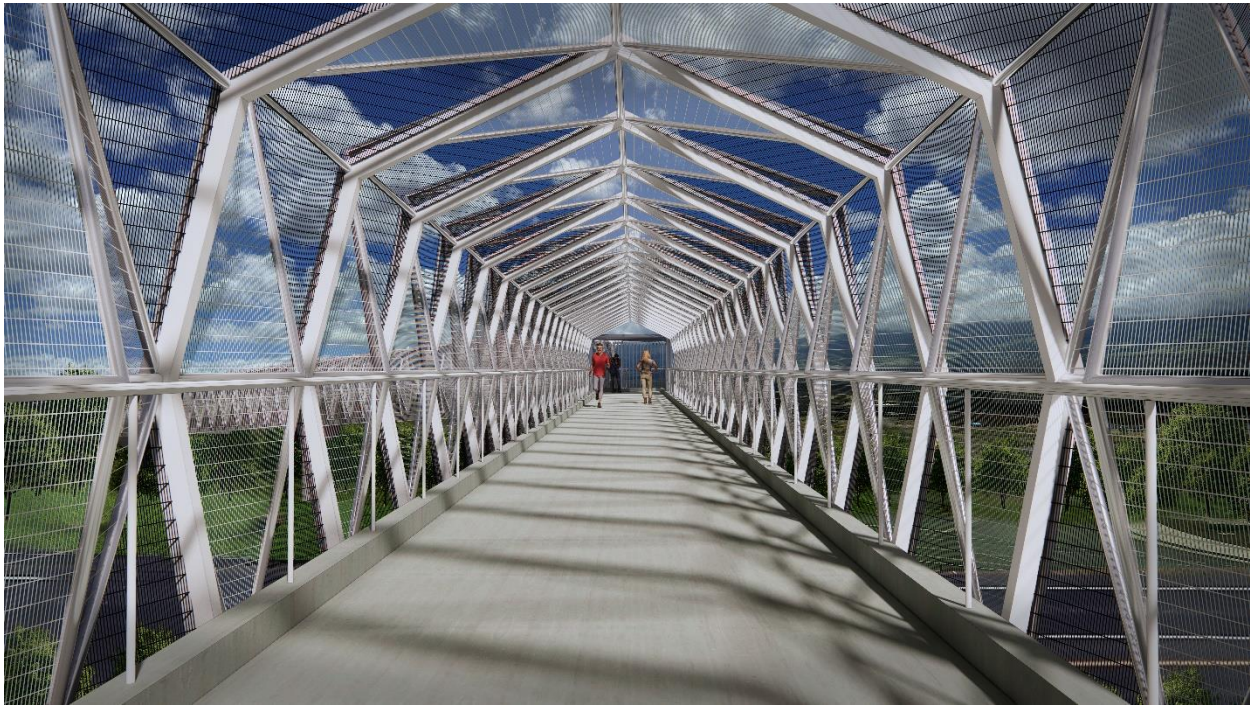
Figure 2-2 Proposed Pedestrian Overpass Bridge Design
