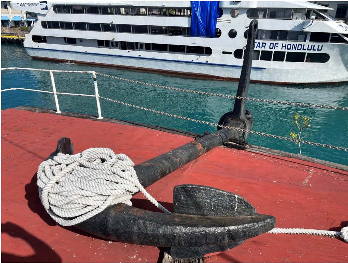
Figure 10: The patent sheet anchor on the forecandle head deck, port side.
