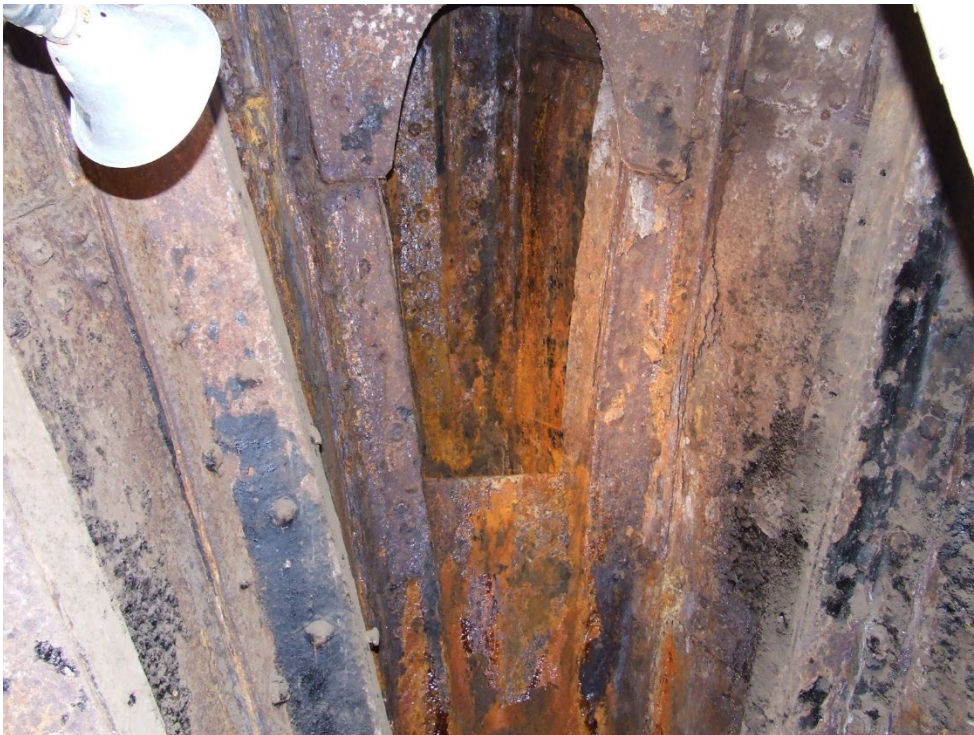
Stern casting, inboard face showing much wastage.
