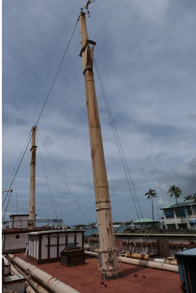
Figure 3: Condition and status of standing rigging for the mizzen and jigger masts (Joseph Lombardi).
