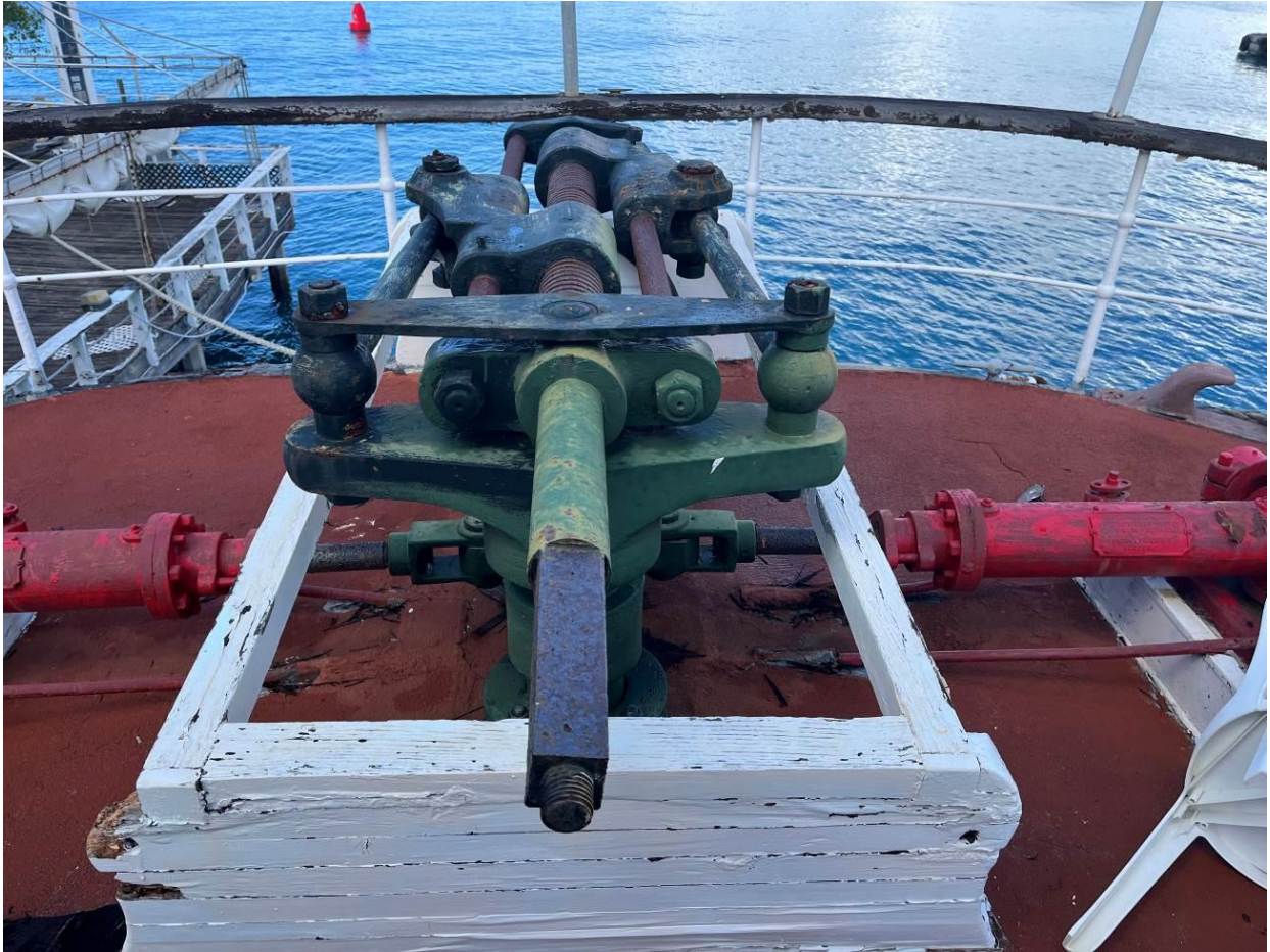
Figure 5: This is the front of the patent steering apparatus, showing where the wheel, which also remains on the ship, and is stowed below, would have been fitted.
