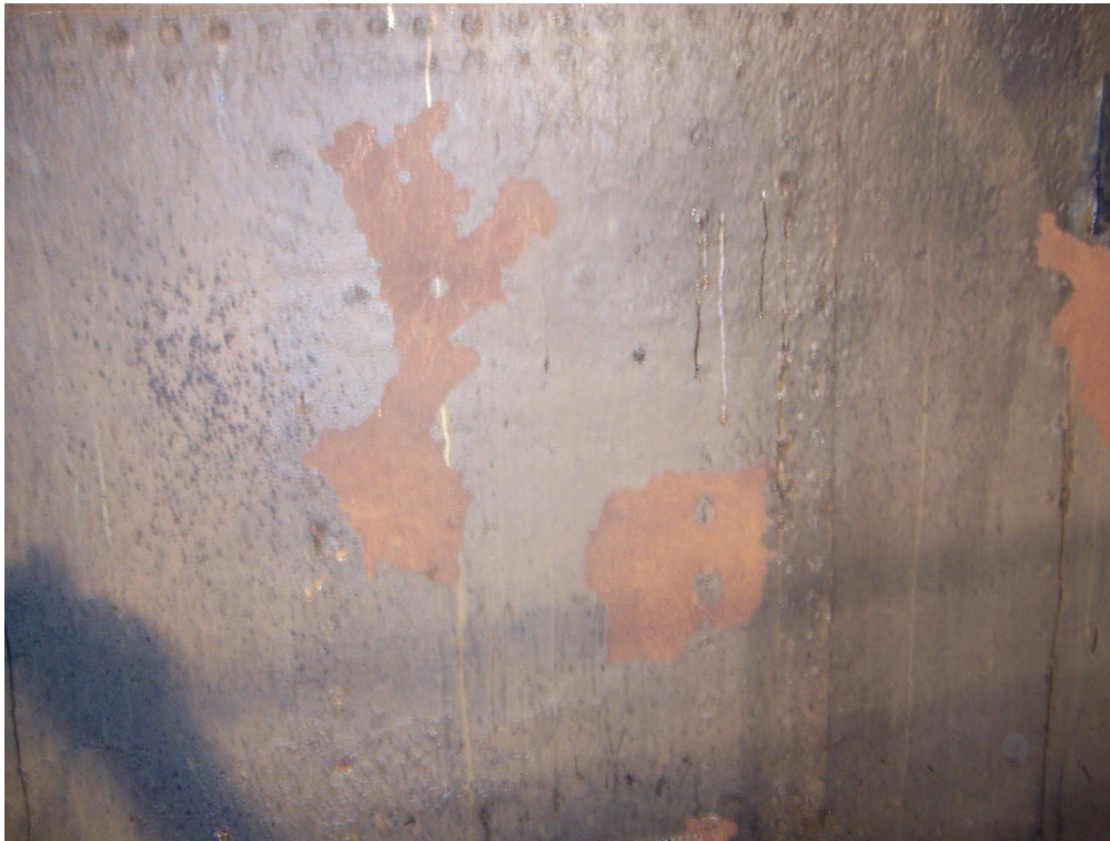
New paint system failure on bulkhead.
