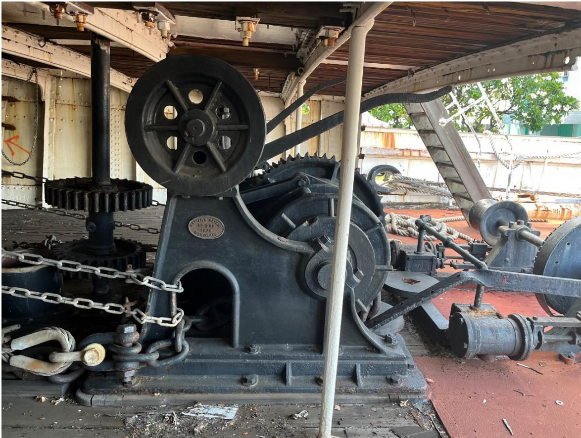
Figure 6: This is the Napier Patent Windlass of the ship; it is original and is in very good condition.
