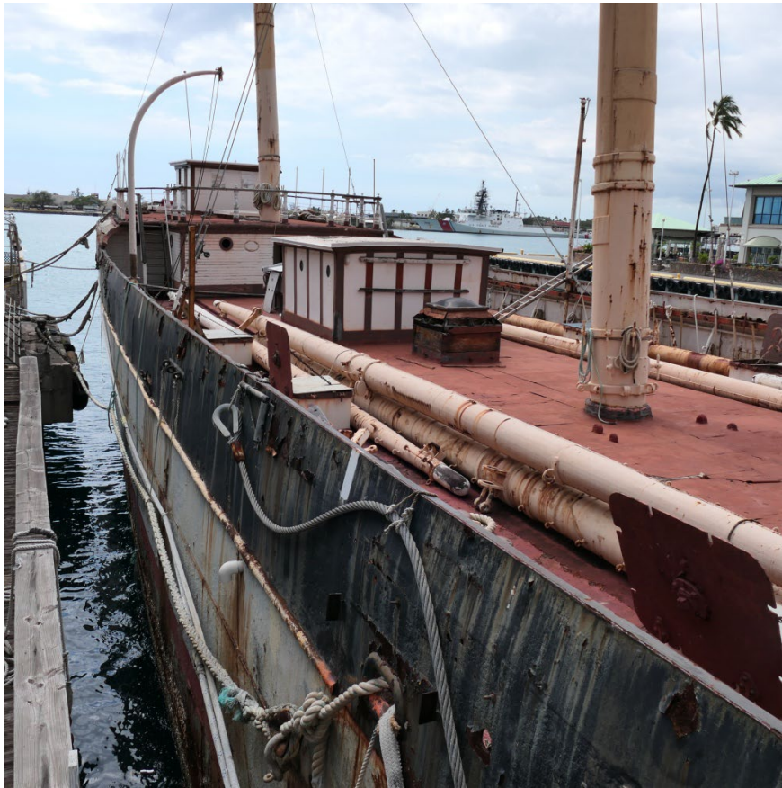
Looking aft at FOC mooring system showing lack of fendering.
