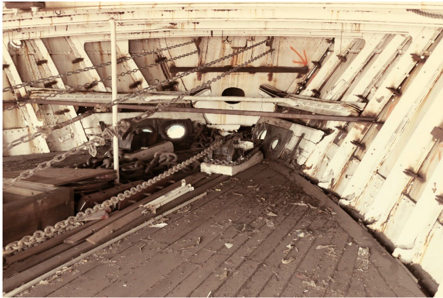
Forecastle showing chains and transverse steel bars supporting collision bulkhead and shell plating to transverse frames.
