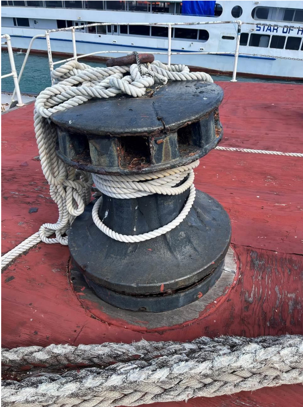
Figure 9: The capstan on the forecastle head deck.
