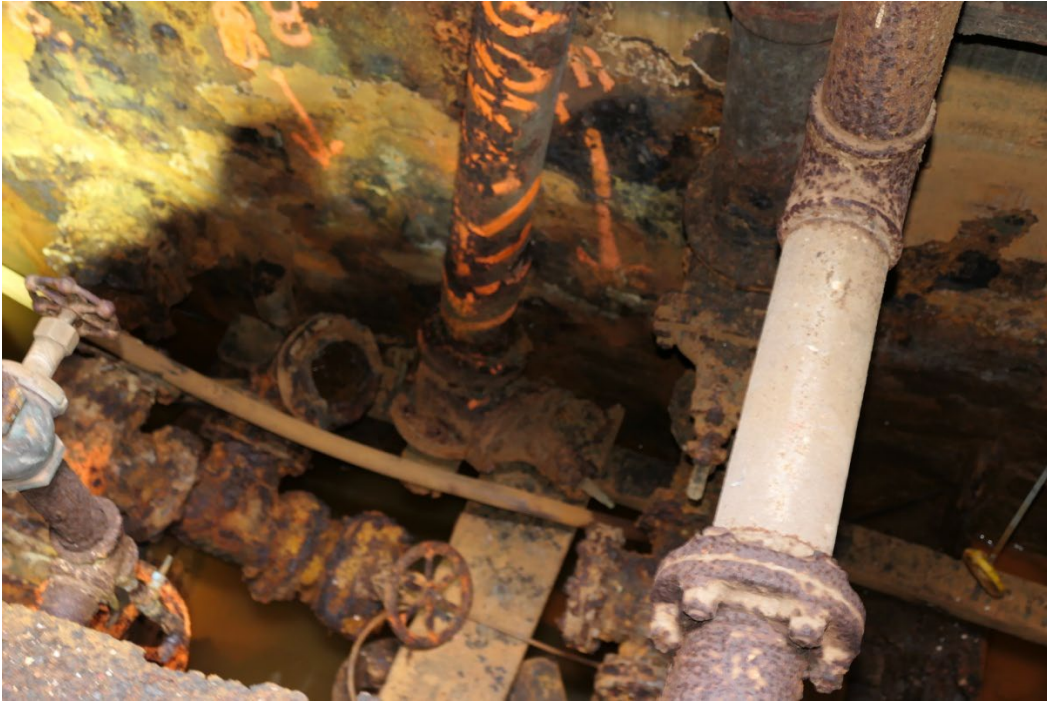
Piping manifold aft of dual steam pumps, showing broken sections in bilges,
