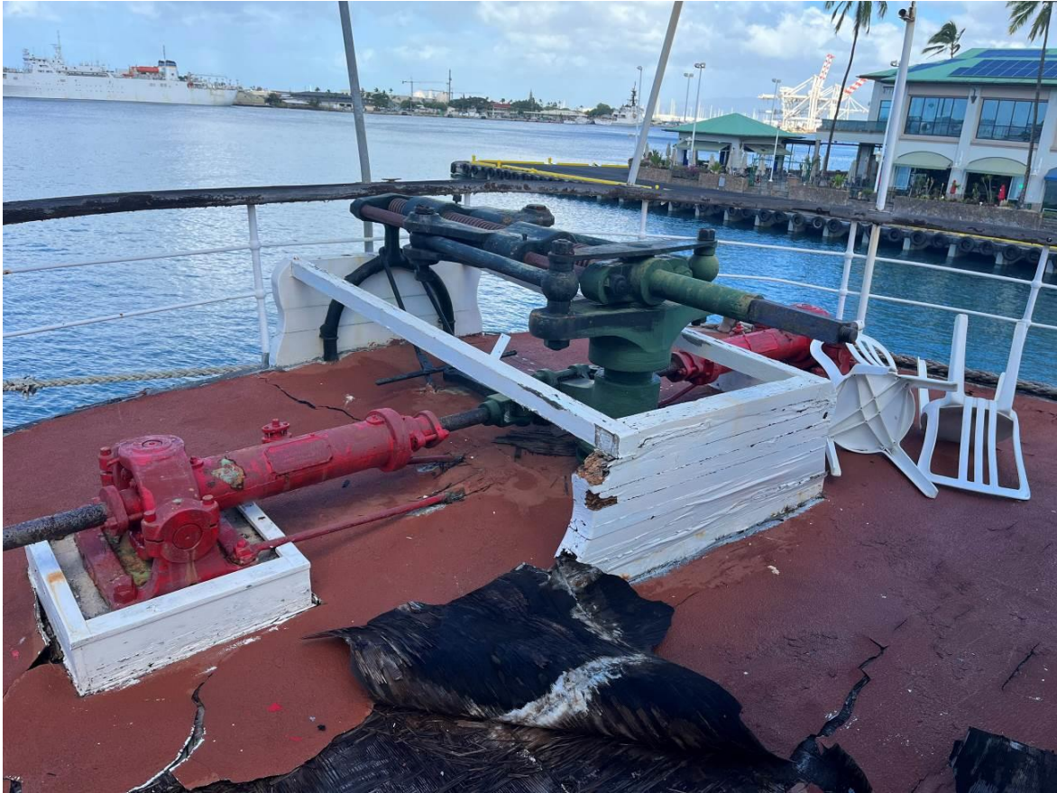
Figure 4: This is the ship's patent steering apparatus. It was covered by a wooden (teak) box that is on the ship but in poor condition. The wheel was attached to it. The red cylinders are oil-filled "brakes" used to assist in handling the helm. There is a solid shaft that runs through the deck and down to the rudder.
