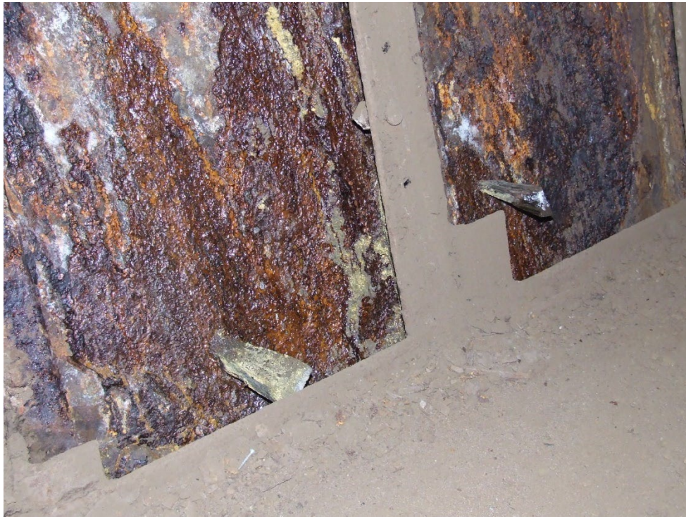
More wasted plating with wooden plugs. Notice separation of shell plating from frames.
