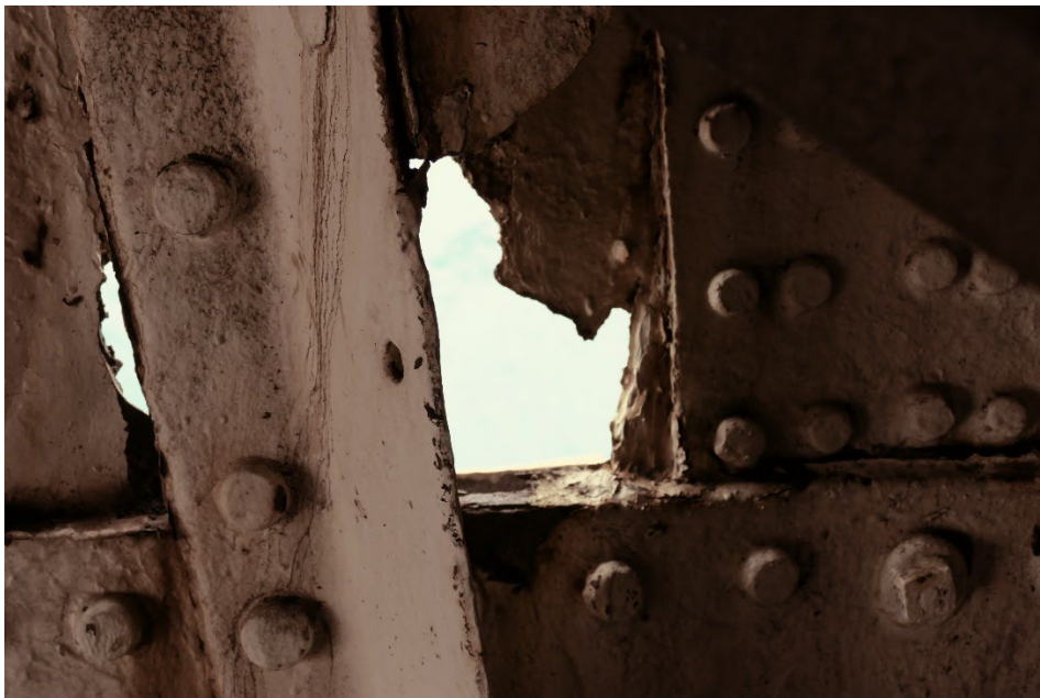
Holed shell plating to port showing dilapidated transverse frame and wasted rivets at bow.
