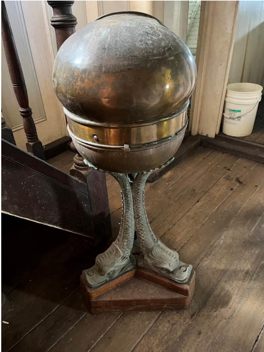
Figure 2: This is the ship's binnacle, which was located on the aft (poop) deck next to the helm. It holds the ship's compass.
