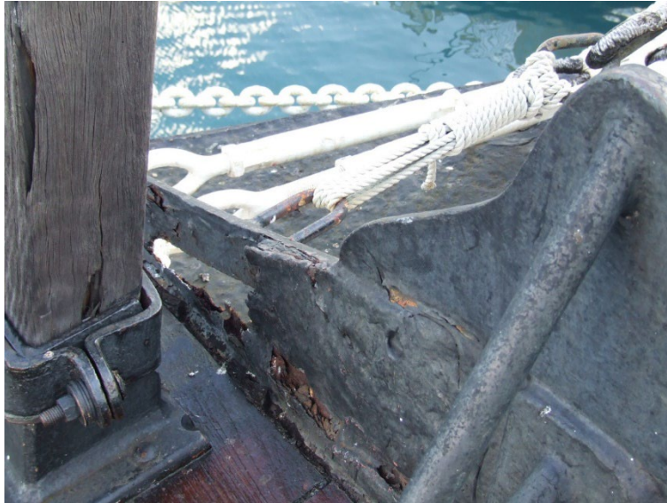
Corrosion of the deck and margin plates is evident in this picture. Notice eyebolt supporting bowsprit guywire lacings.
