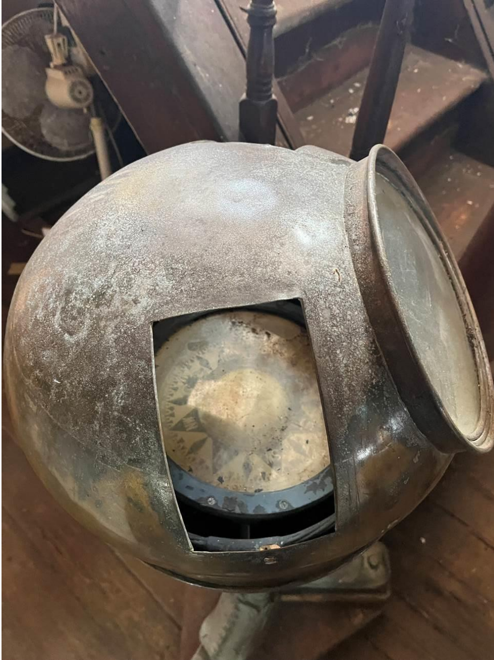
Figure 3: The ship's compass remains inside the binnacle. This is a valuable artifact.
