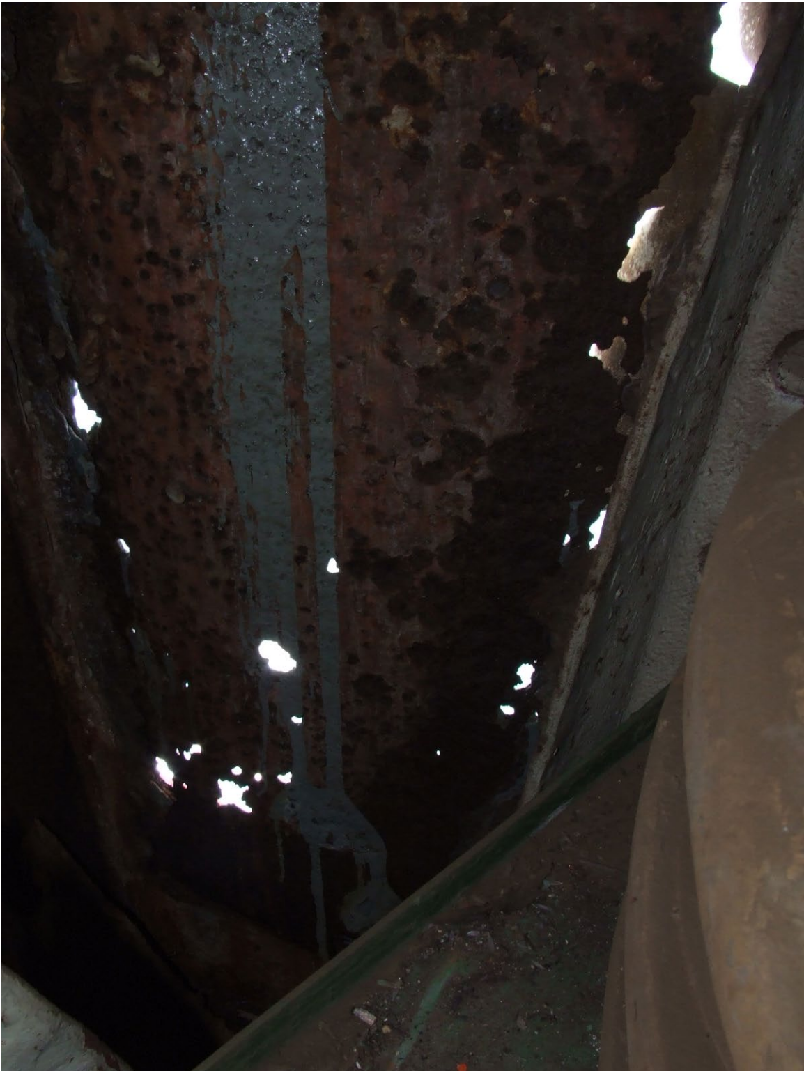
Holed shell plating just above waterline to port of stern casting. Nothing left to repair.
