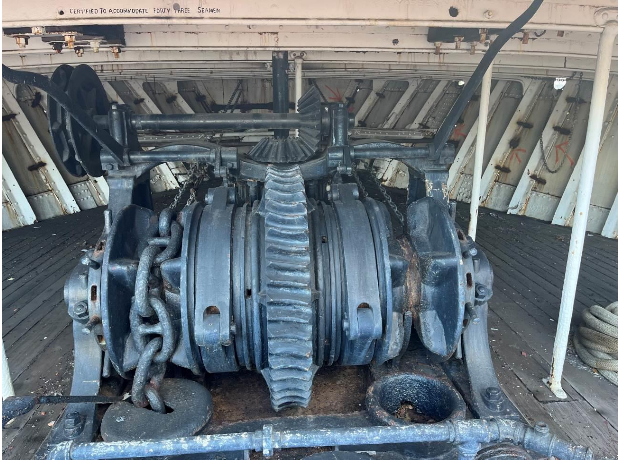
Figure 7: This is the front of the Napier Patent Windlass; it is located in the forecabin head and is bolted to the deck; the gearing includes a connector that runs up to the forecabin head deck that drove the capstan.
