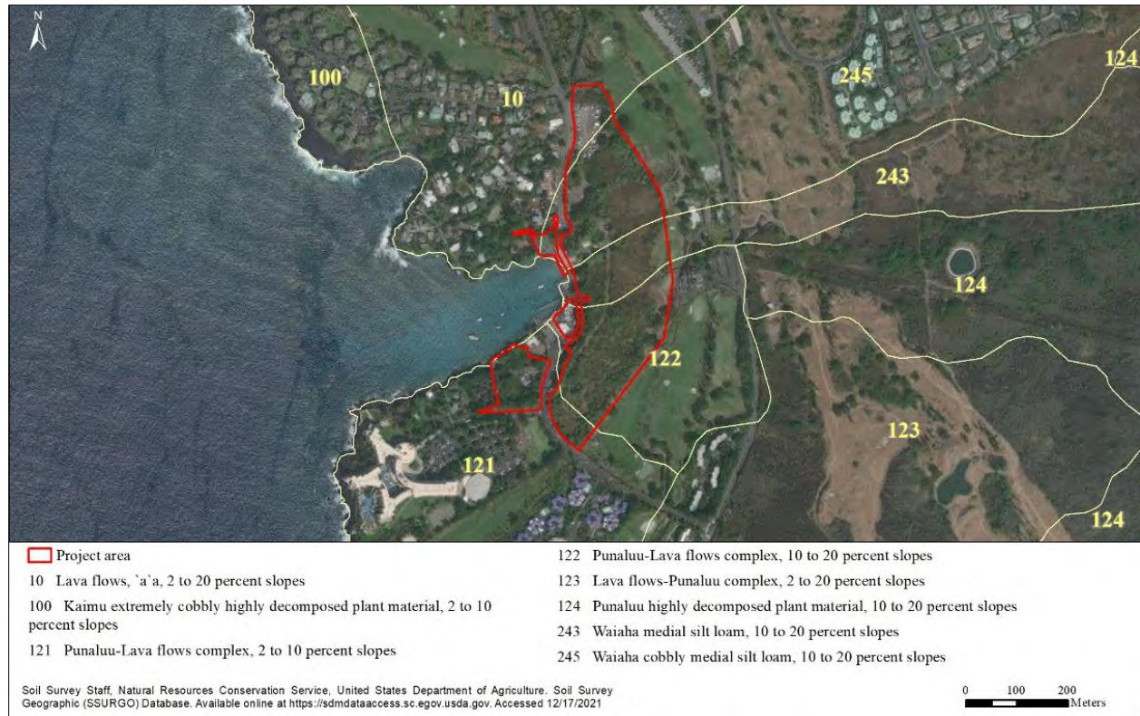
Figure 15. Soils underlying the project area.
