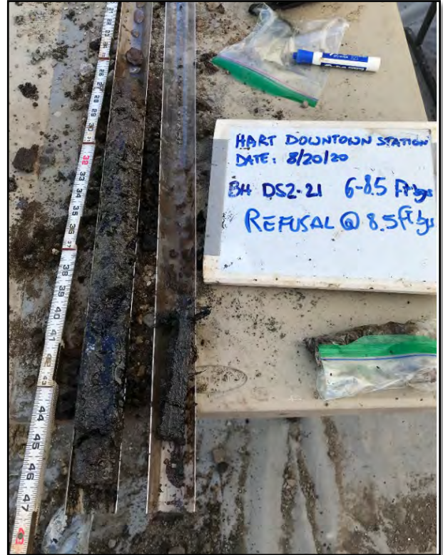
Photo 6: Soil core representative of fill material, with grossly impacted soil (medium black sand) at the bottom.
