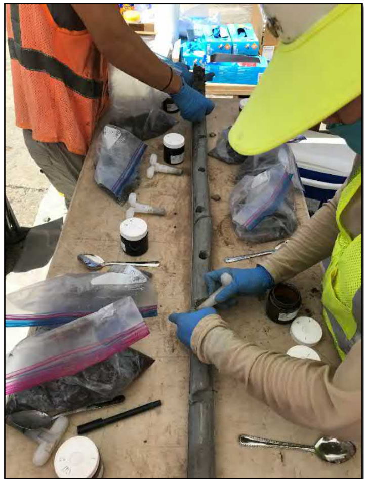
Photo 4: MIS soil sampling activities using dedicated terracoors.
