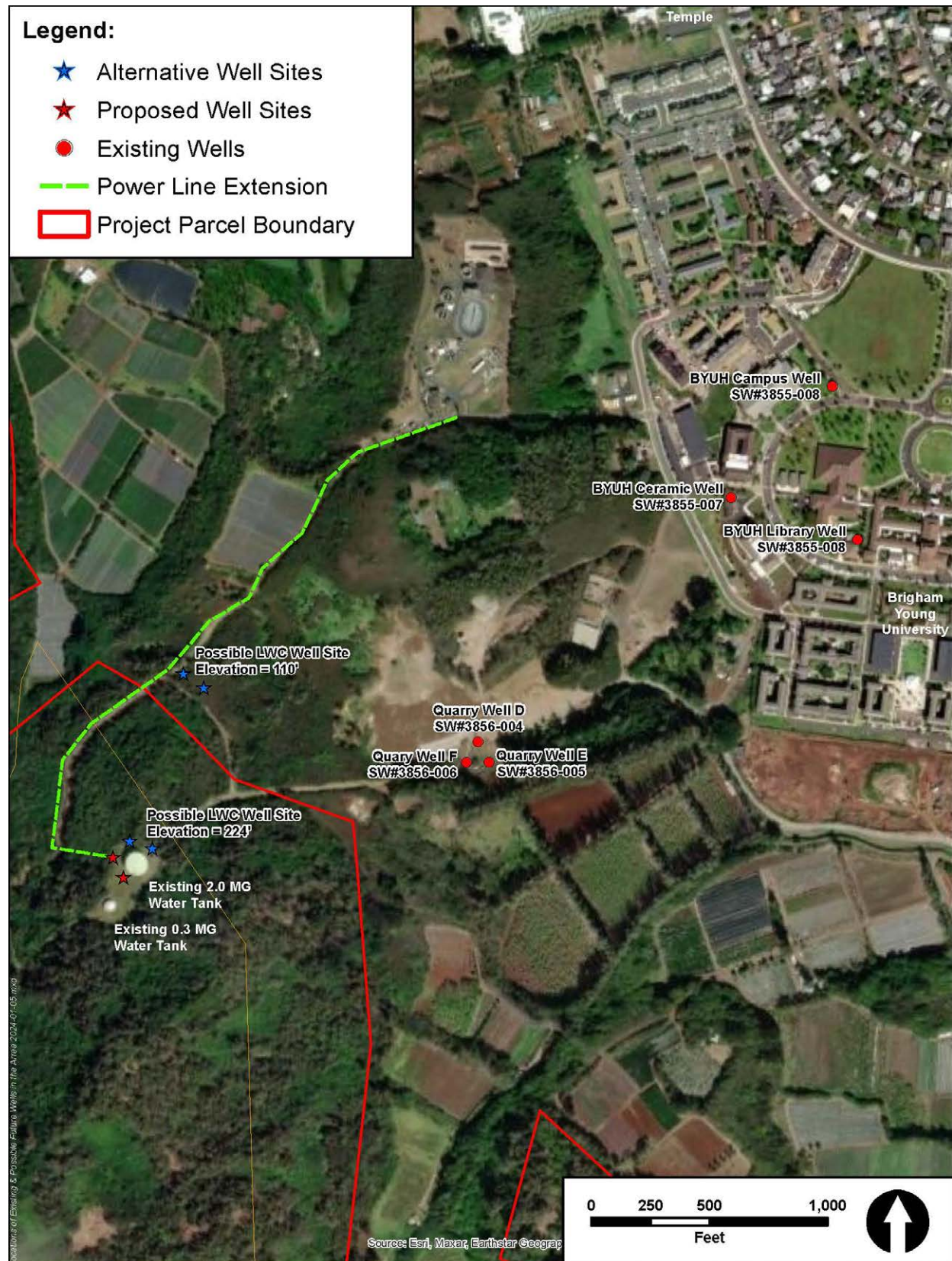
Figure 2-12: Locations of Existing and Possible Future Wells
