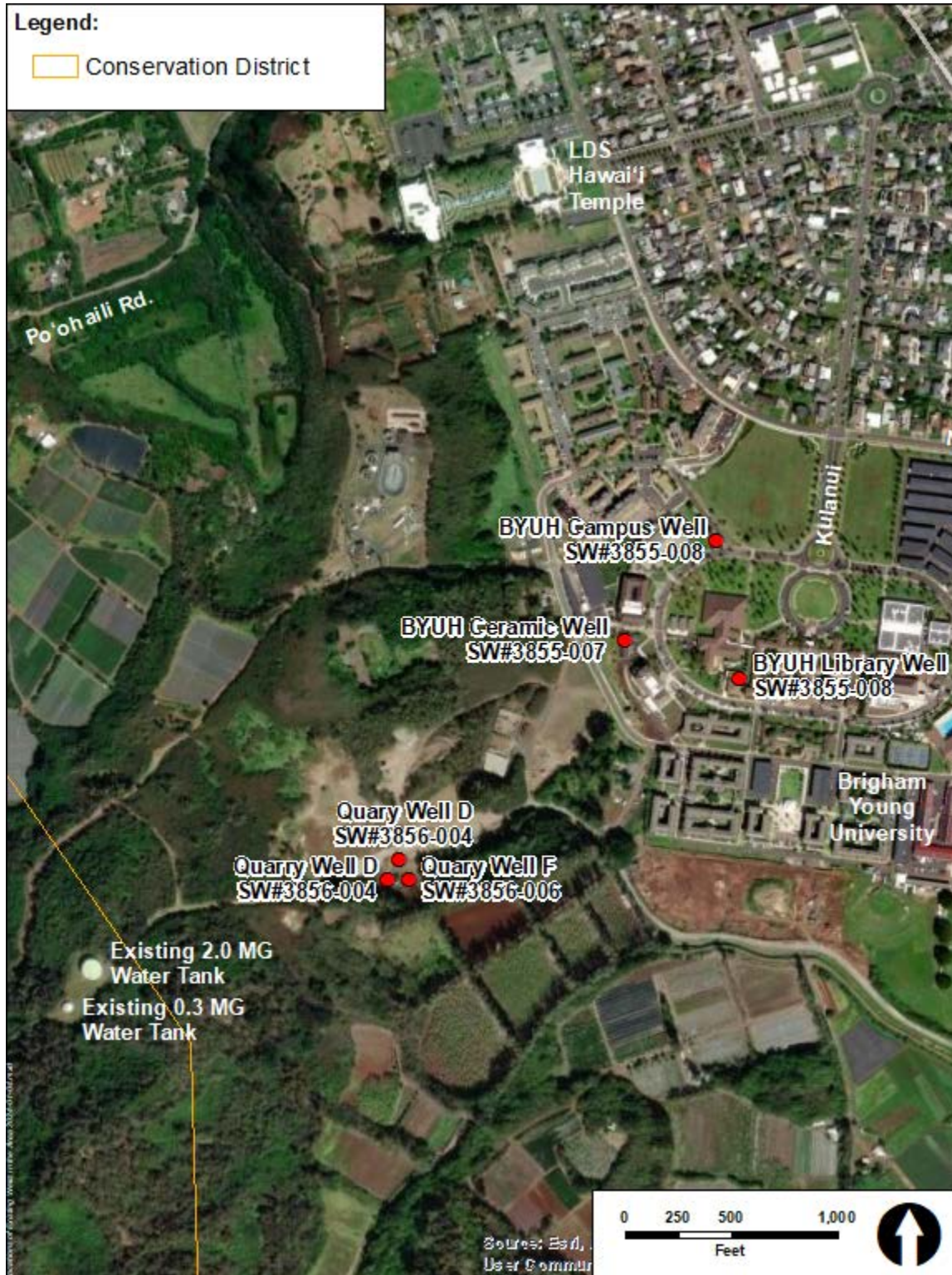
Figure 1-3: Location of Existing LWC Wells and Tanks
