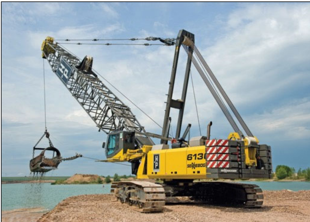
Figure 7-21 Sennebogen 6130 HD duty cycle crawler crane ( www.sennebogen.com )
