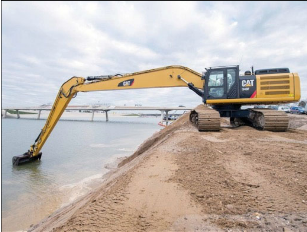
Figure 7-20 CAT 352F LRE long reach excavator ( www.caterpillar.com )
