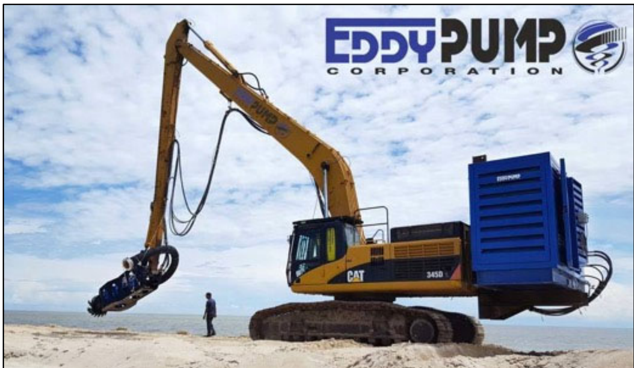
Figure 3-13 Excavator with 10-in dredge pump and power pack (EddyPump ® , 2021)
