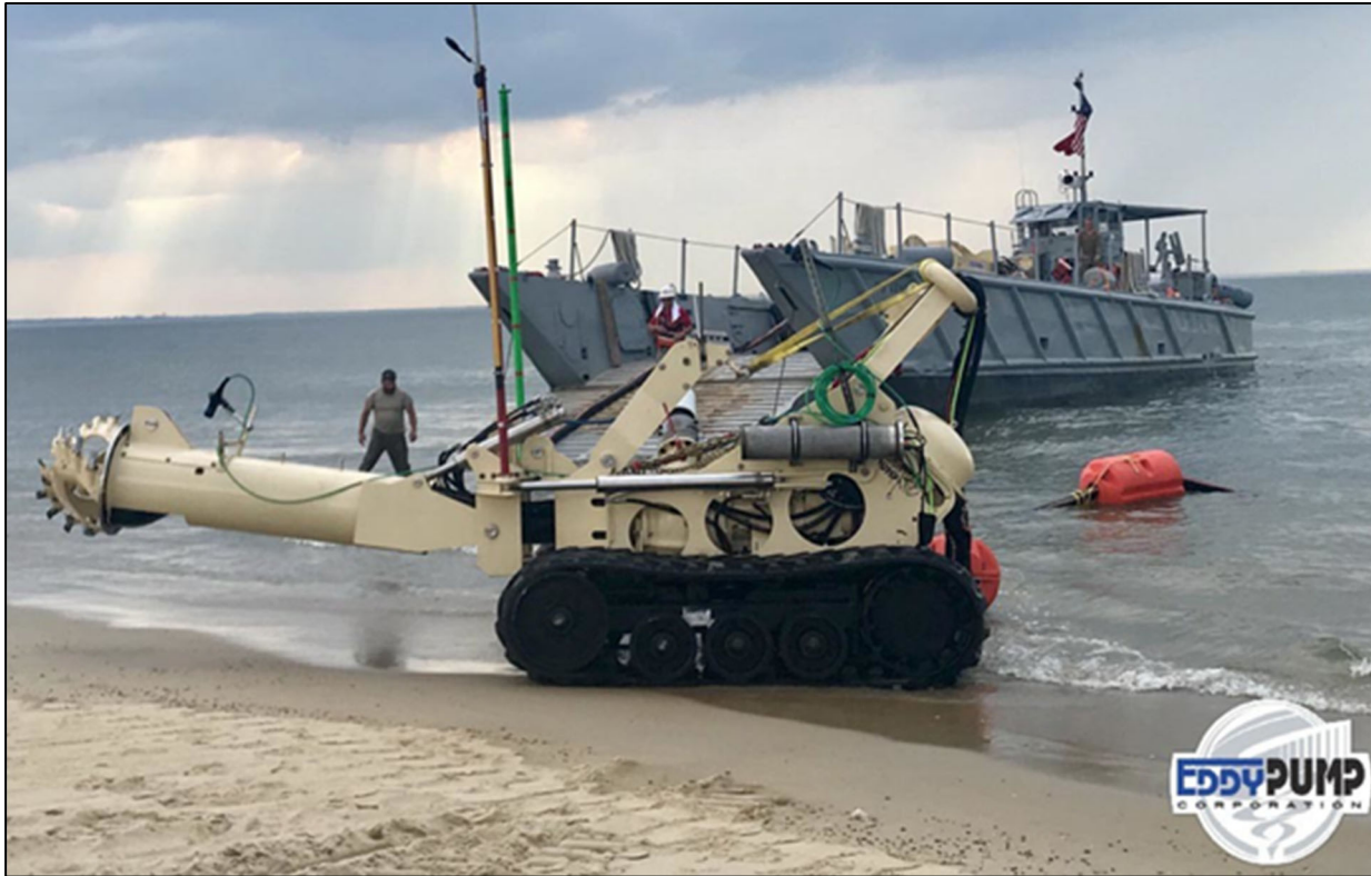
Figure 3-10 Remote Operated Submersible Dredge (Eddy Pump ® , 2021)
