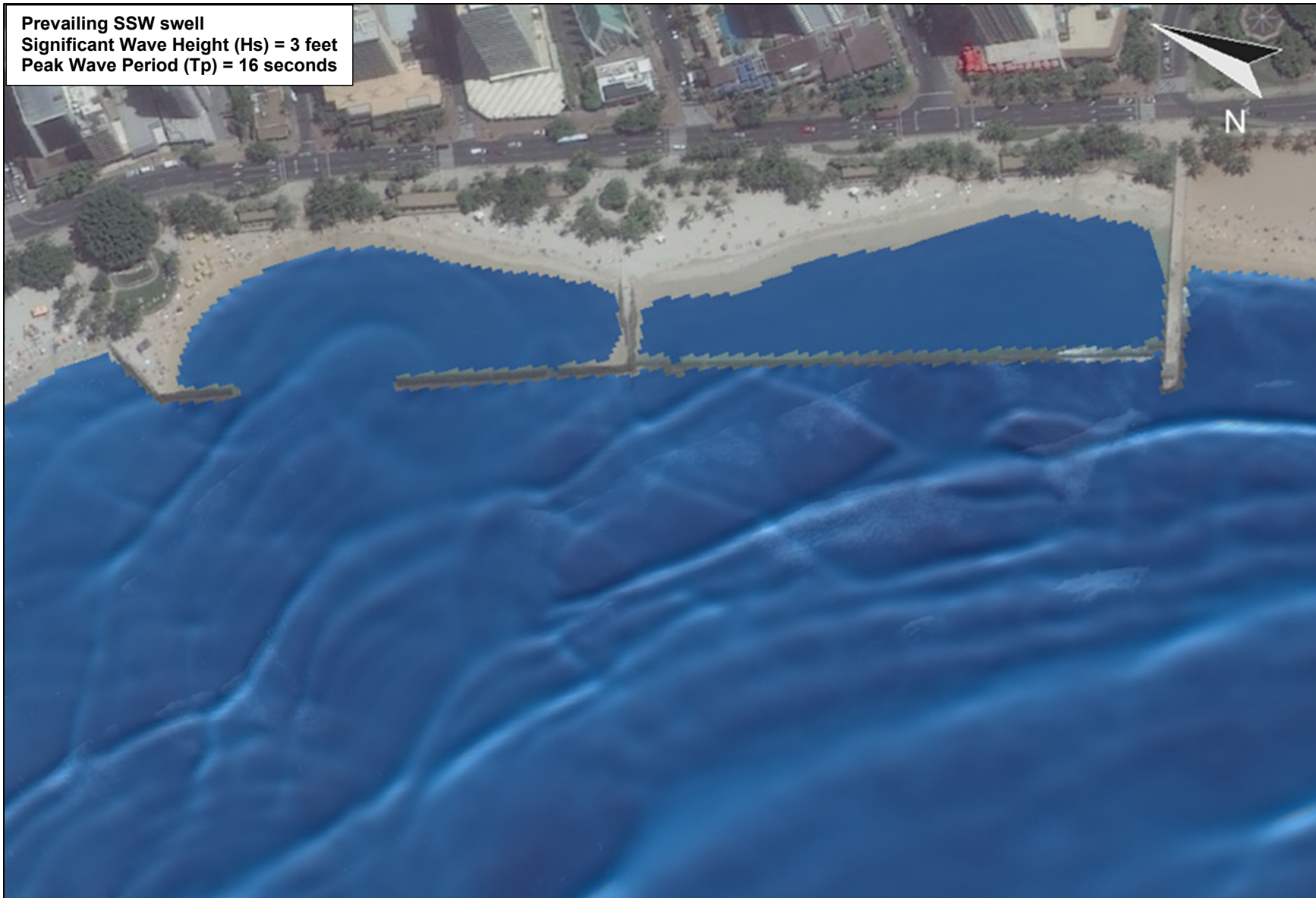
Figure 8-10 XBeach-NH wave pattern for high-prevailing SSW swell – Kūhiō beach sector
