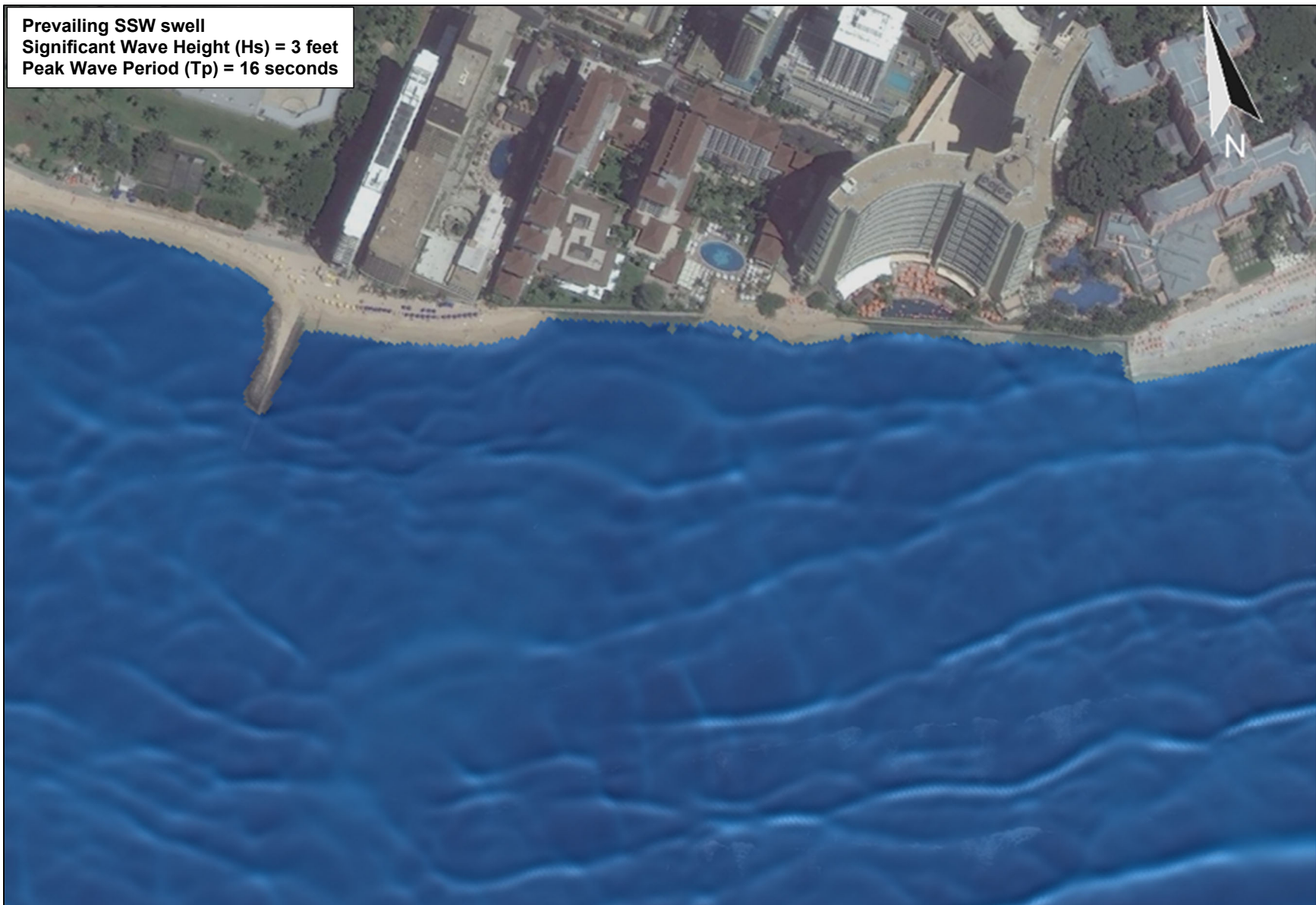
Figure 8-8 XBeach-NH wave pattern for high-prevailing SSW swell – Halekūlani beach sector
