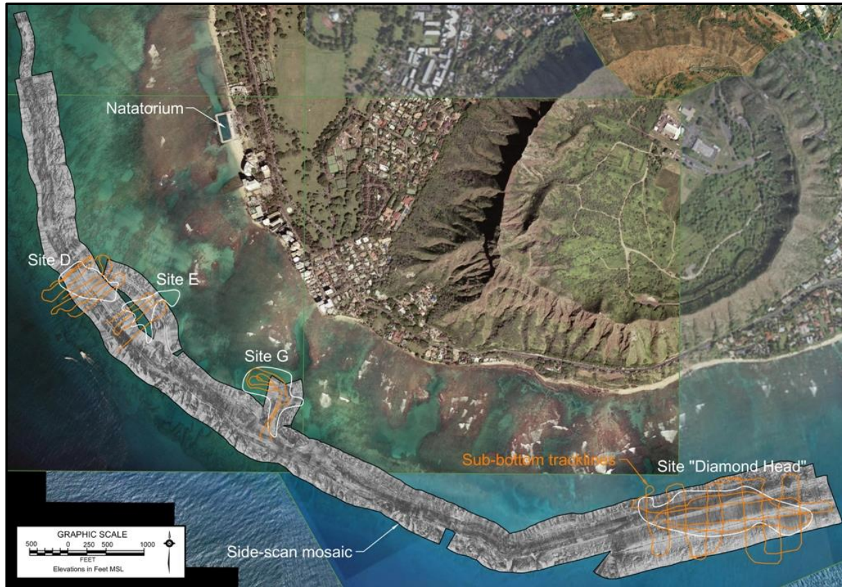
Figure 3-11 Side-scan sonar mosaic and sub-bottom profiler tracklines
