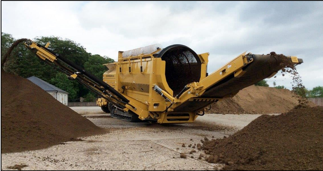
Figure 5-29 Anaconda TD620 Trommel Screen used to separate coarse material
