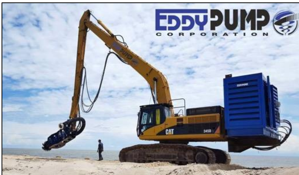
Figure 5-12 Excavator dredge pump attachment with 10-in pump and power pack (EddyPump® Corporation, 2021)
