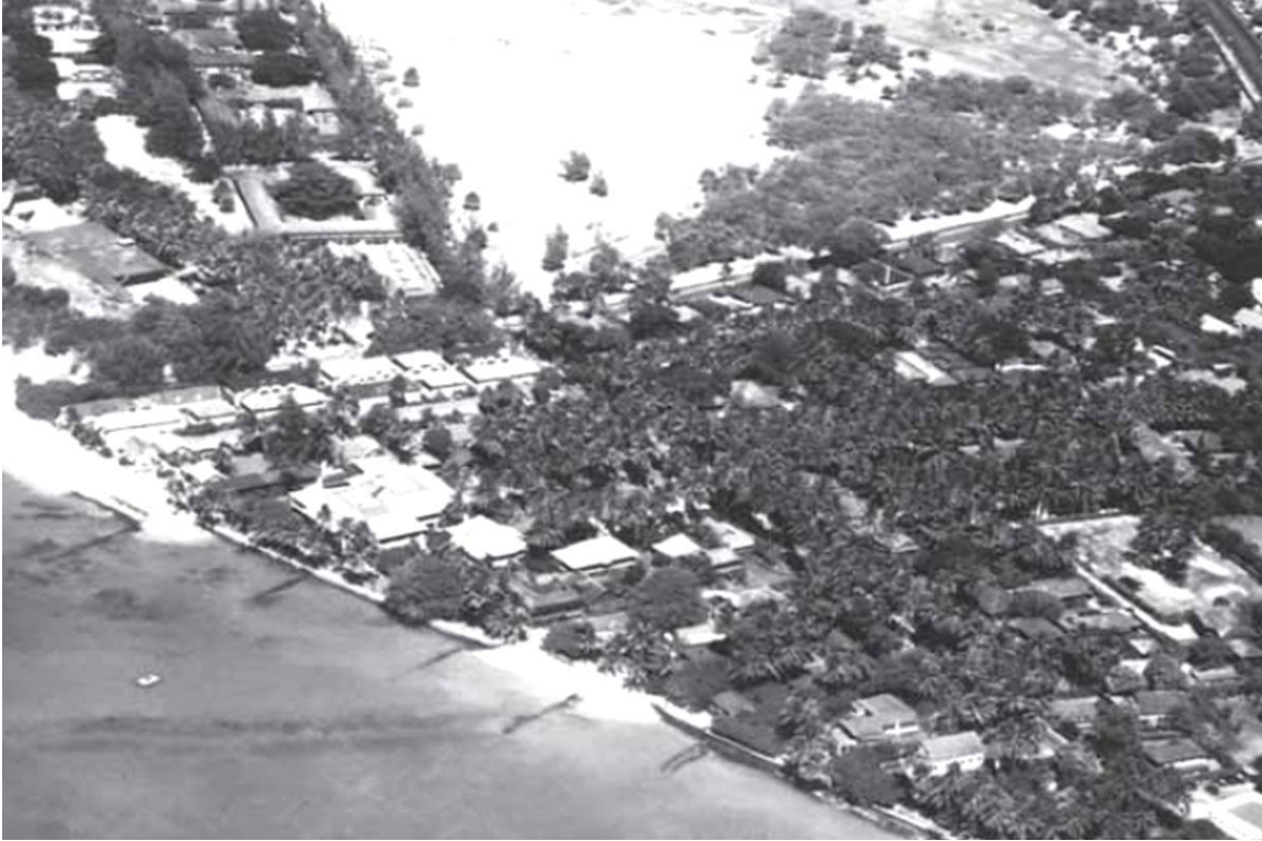
Photo 9. A 1932 aerial photograph showing groins along the shoreline of the Halekūlani sector. Reproduced from Wiegel 2008:Figure 19.
