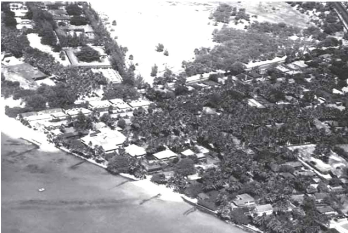
Photo 10. A 1932 aerial photograph showing groins along the shoreline of the Halekūlani sector (source: Wiegel 2008:Figure 19).
