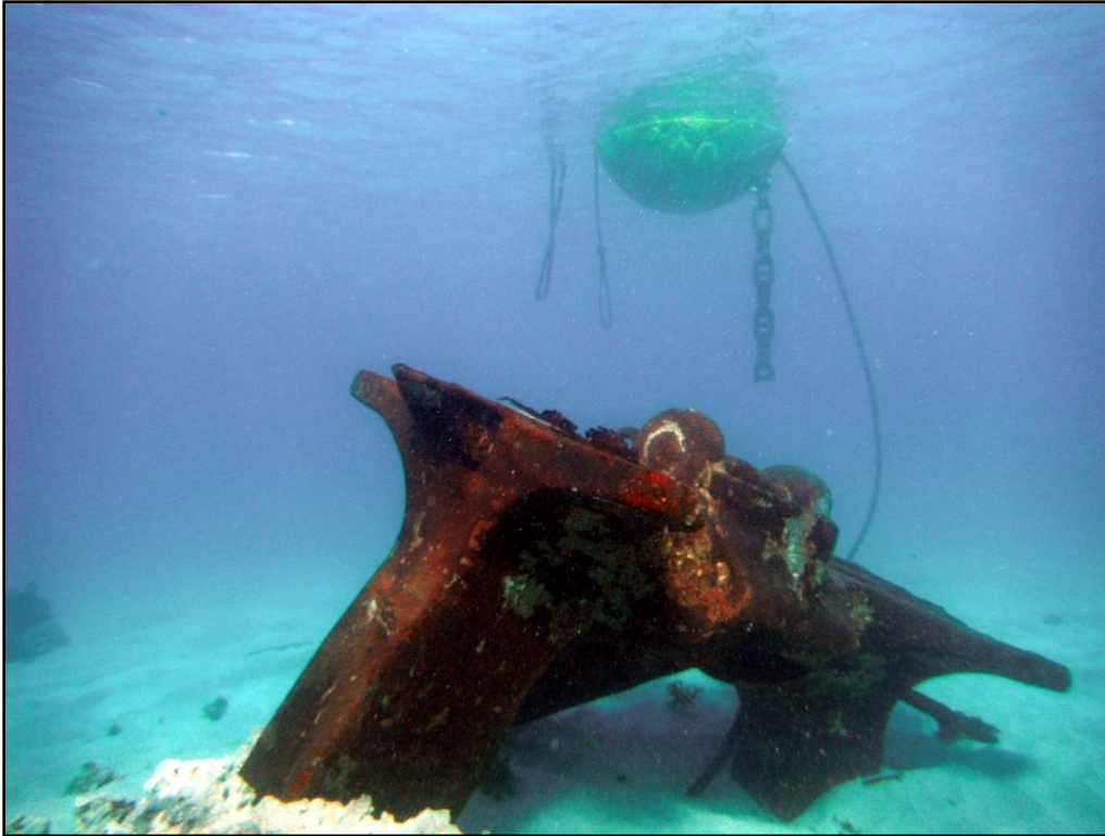
Figure 5-1 Example: Anchor and Anchor Float used in the 2012 Waikiki Beach Maintenance Project.
