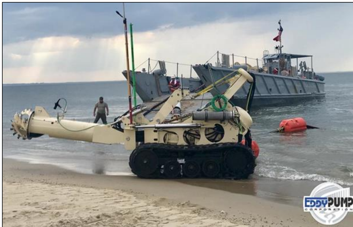
Figure 5-9 Remote Operated Submersible Dredge (Eddy Pump, 2021)
