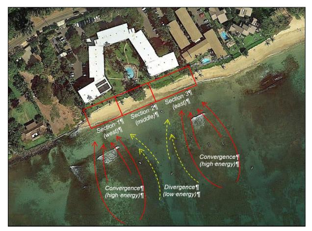
Figure 4-2 Wave dynamics along the KAN shoreline
