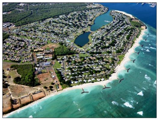
Figure 5-5 Beach restoration with T-head groins at Iroquois Point, Oahu (2017)
