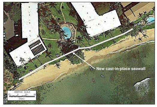
Figure 5-19 Conceptual plan view of a new cast-in-place seawall at KAN
