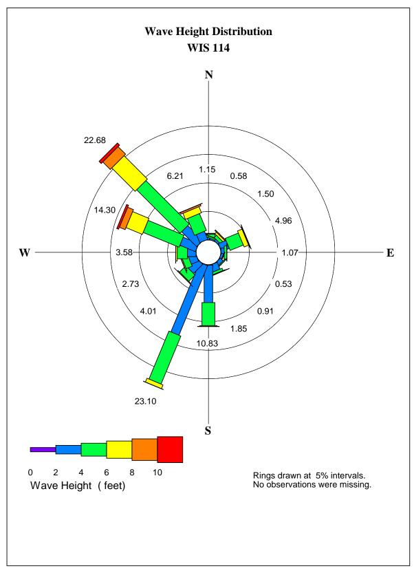
Figure 3-3 Wave height distribution (WIS Station 114)
