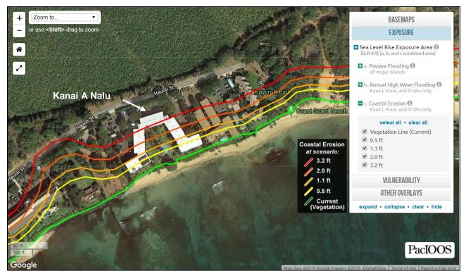
Figure 2-5 Coastal erosion with 0.5 to 3.2 feet of sea level rise (PacIOOS)
