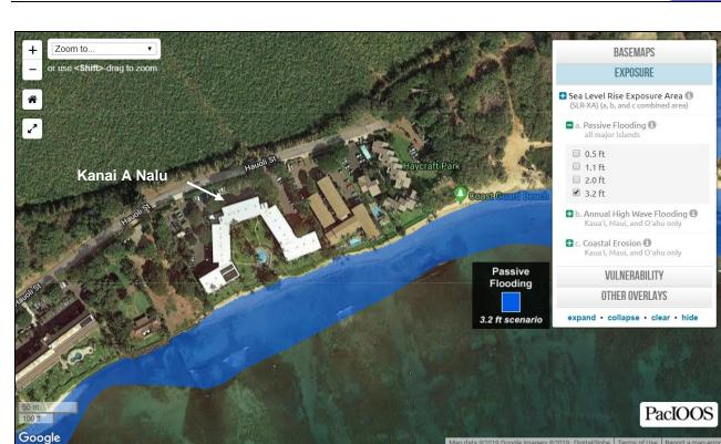
Figure 2-3 Passive flooding with 3.2 feet of sea level rise (PacIOOS)
