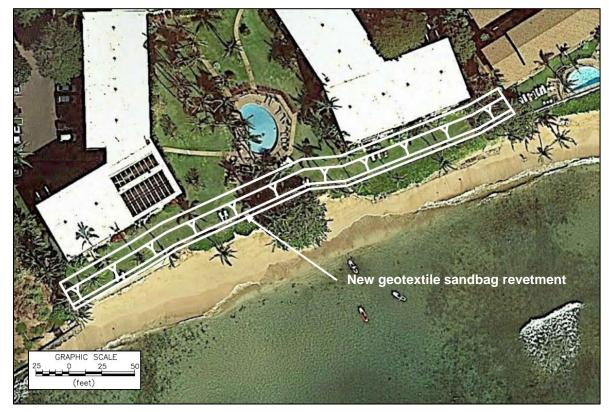
Figure 5-13 Conceptual plan view of a geotextile sandbag revetment at KAN
