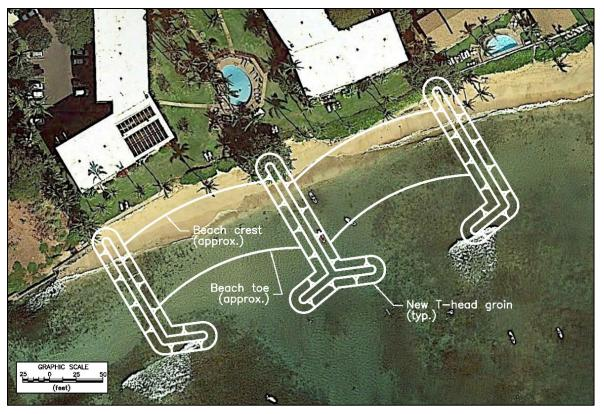
Figure 5-6 Small-scale beach restoration with T-head groins
