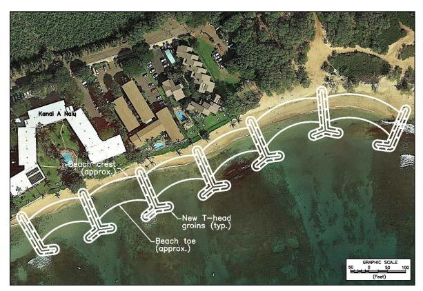
Figure 5-7 Large-scale beach restoration with T-head groins
