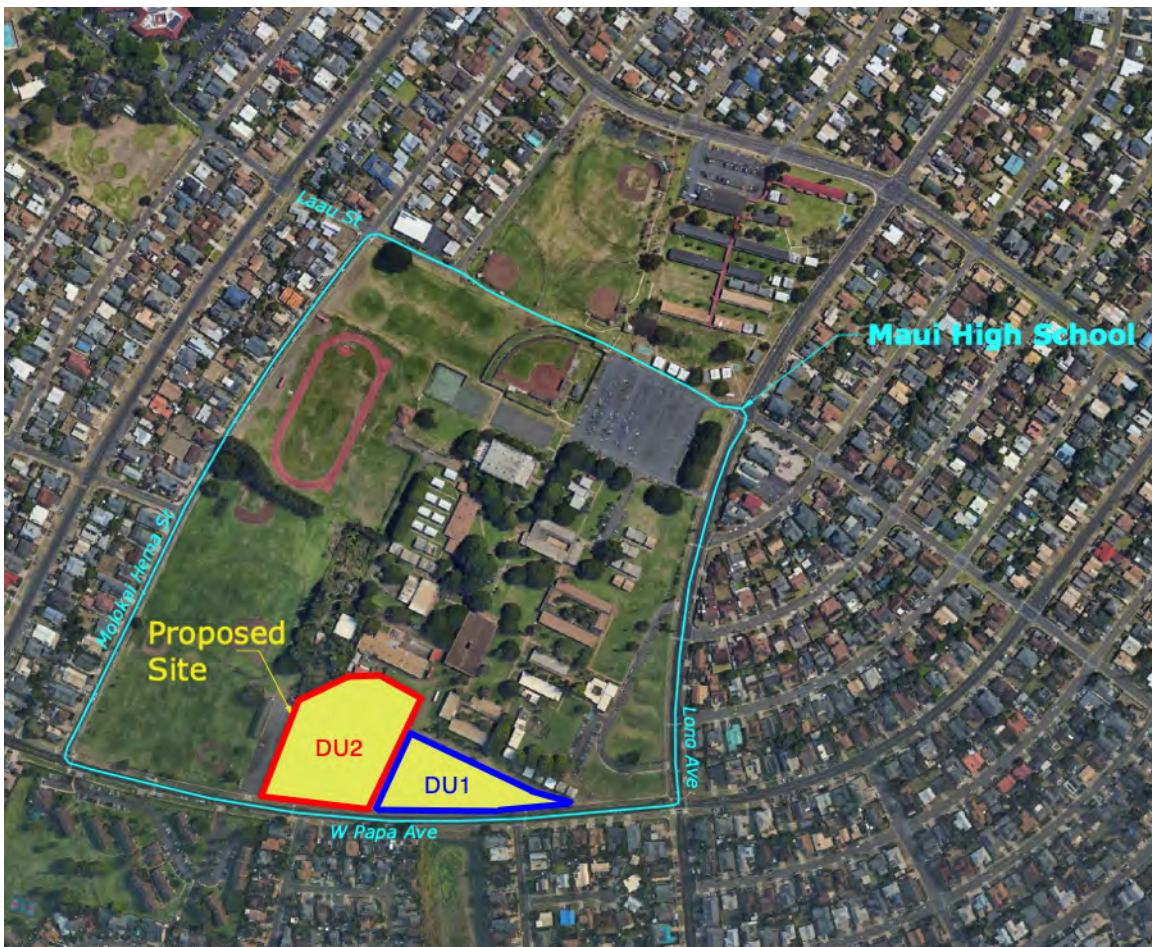
Figure 1: Schematic of the Decision Units locations at Maui High School. Soil increments were obtained from depths of 1 - 6 inches below the ground surface of native soil.
