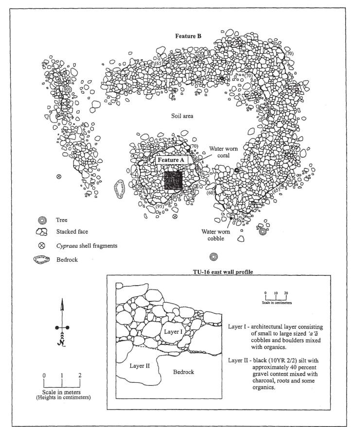
Figure 36. SIHP Site 23677 plan view and TU-16 profile.
