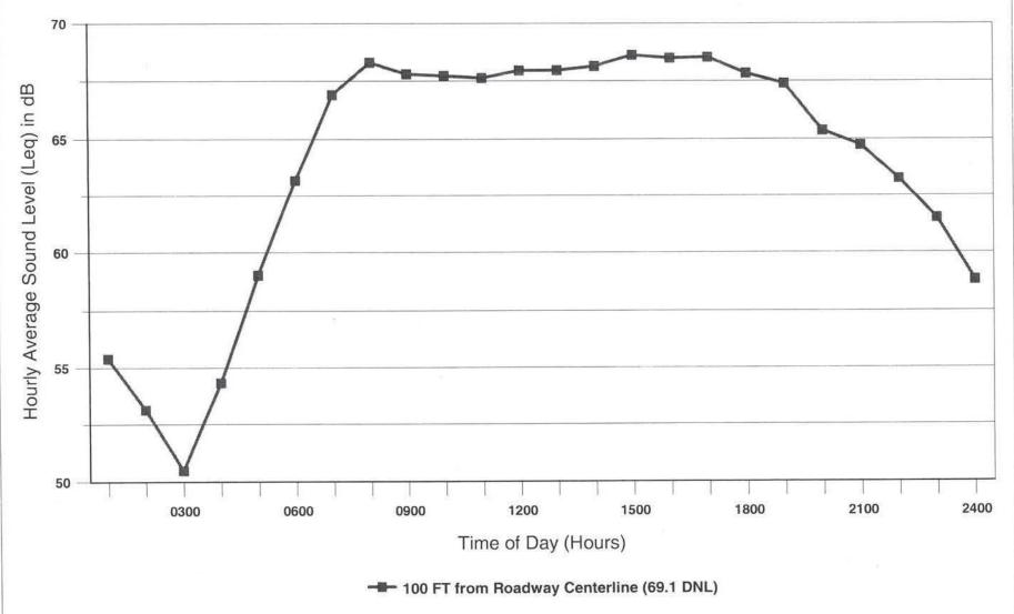
FIGURE IV-6 HOURLY TRAFFIC NOISE LEVELS VS. TIME OF DAY STA. B71001110078; KUAKINI HWY. BETWEEN HUALALAI RD. AND ONI ONI ST.; JANUARY 10, 2019 Hourly Average Sound Level (Leq) in dB Time of Day (Hours)
