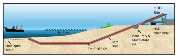
Figure 1-4. Typical HDD Profile
