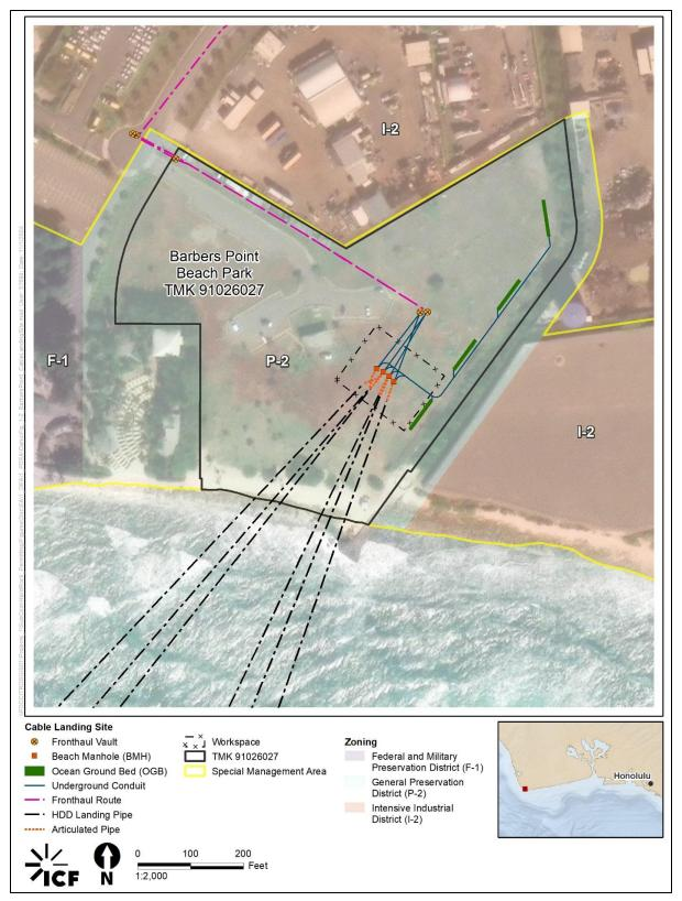
Figure 6. Site plans for the proposed Barbers Point Cable Landing Site for the O'ahu Subsea Cable Telecommunications Project (courtesy of ICF International, 2024).
