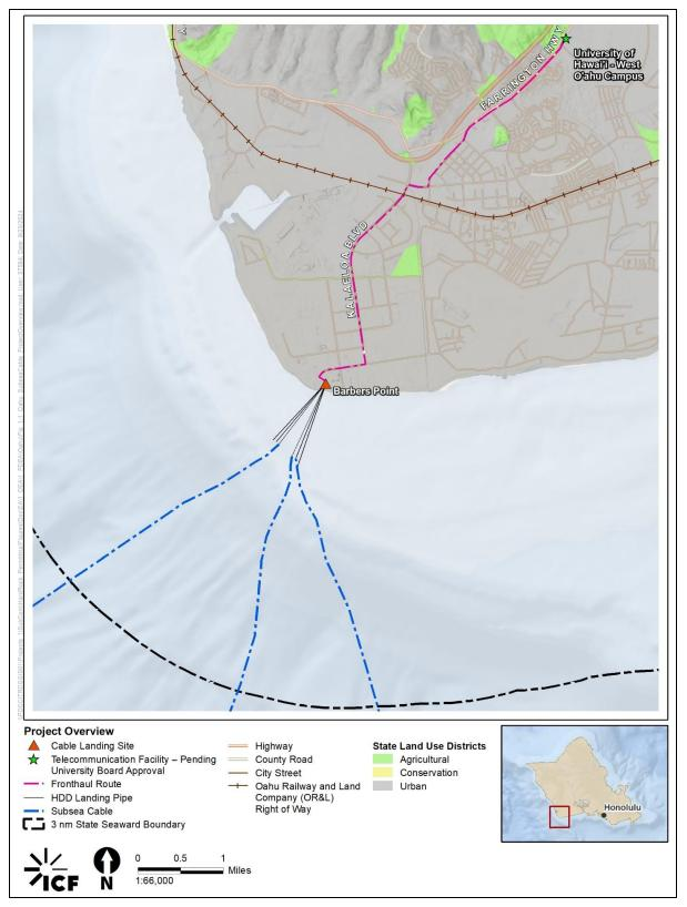
Figure 7. Site plans for the proposed O'ahu Subsea Cable Telecommunications Project (courtesy of ICF International, 2024) (base map: Esri 2024).
