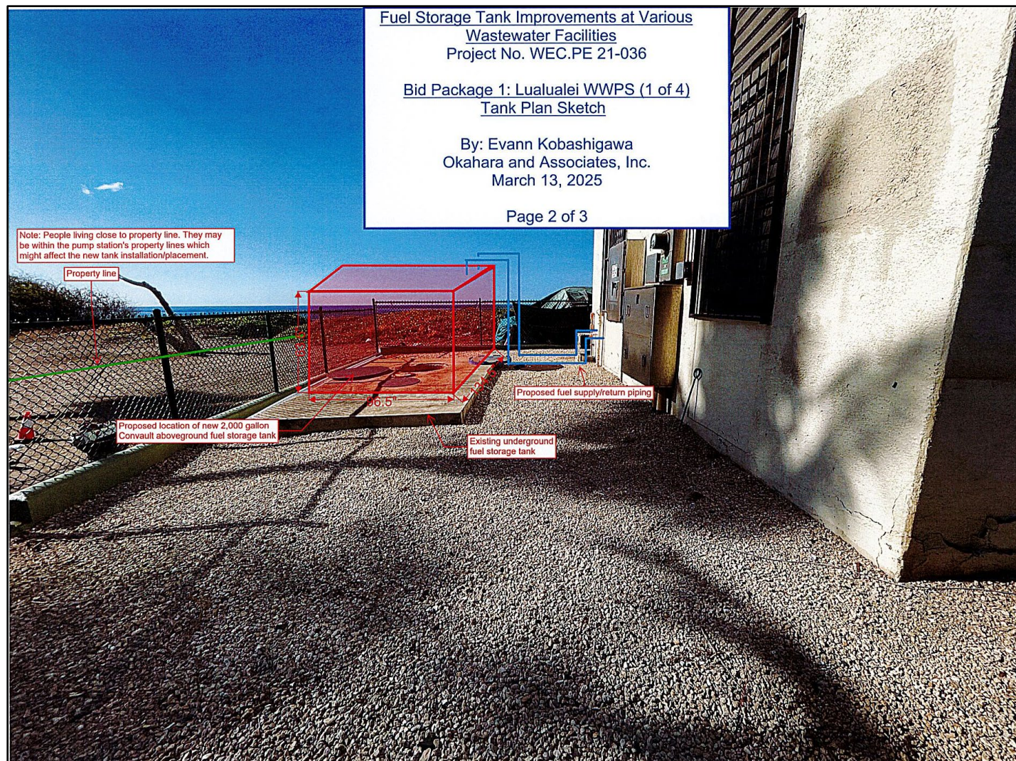
Figure 5. Photograph of the Lualualei WWPS Improvements project showing the proposed location of a new 2,000-gallon Convault aboveground fuel storage tank and the proposed fuel supply/return piping (Okahara and Associates, Inc.; courtesy of client)
