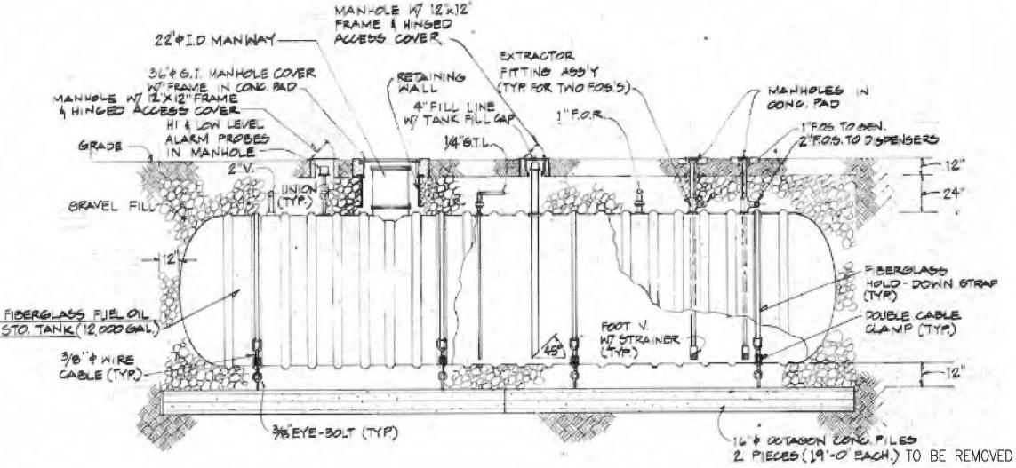
1. UHH SHALL EMPTY THE FUEL TANK AS MUCH AS POSSIBLE AND CONTRACTOR SHALL EMPTY THE REMAINING 100 GAL. OR LESS ON THE FUEL TANK PRIOR TO REMOVAL
