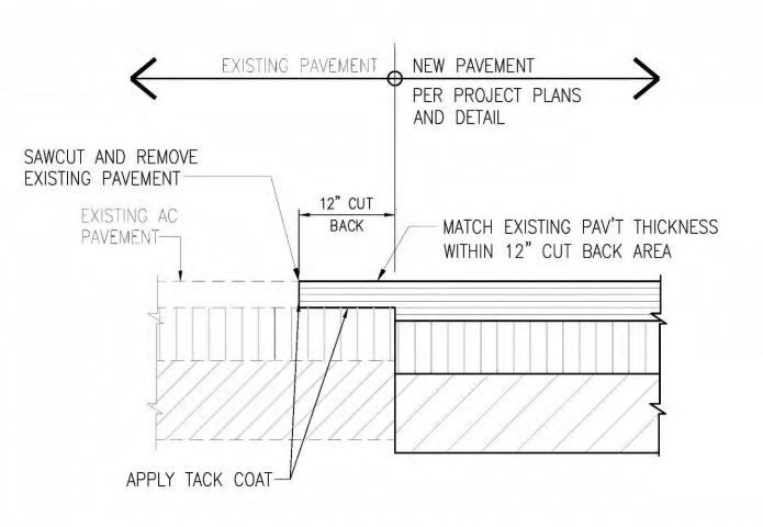
DISTURBED AGGREGATE BASE BELOW EXISTING PAVEMENT SHALL BE RE-COMPACTED PRIOR TO PAVING. FILLING OF ANY VOIDS IN AGGREGATE BASE SHALL BE CONSIDER INCIDENTAL TO THE WORK.
