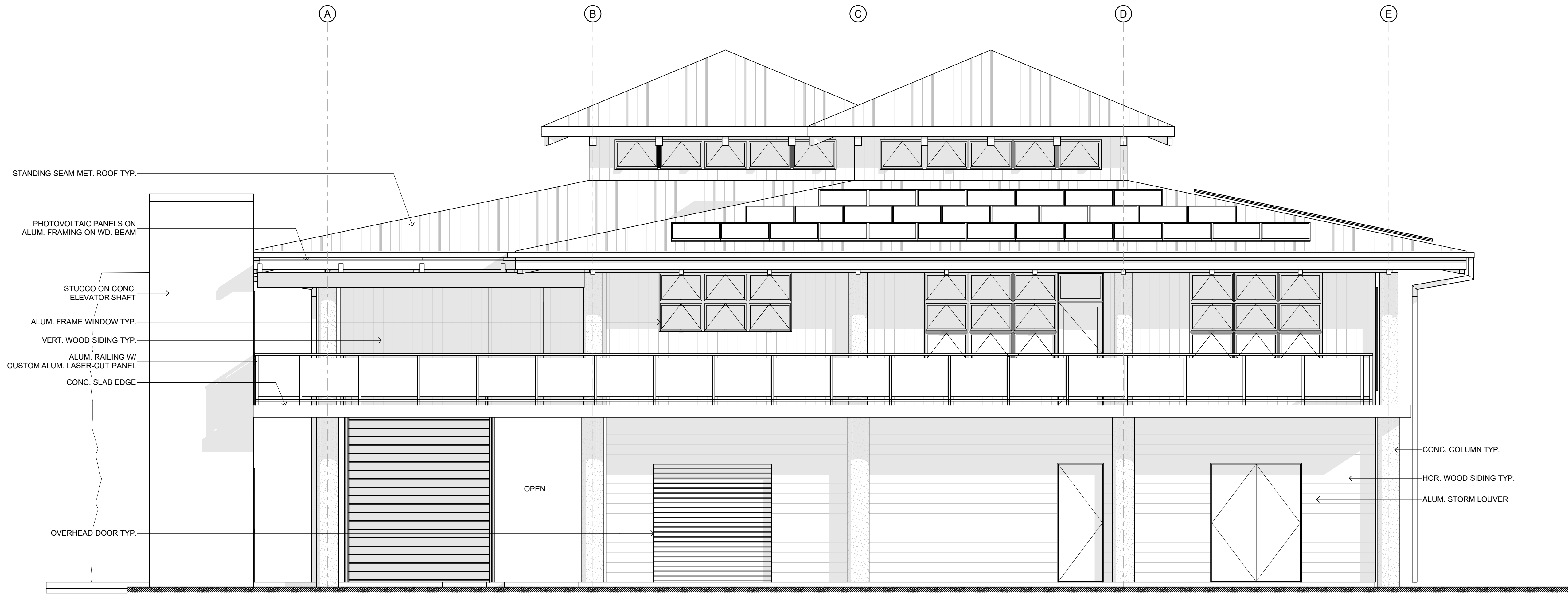
2 WEST ELEVATION SCALE: 1/4" = 1'-0"
