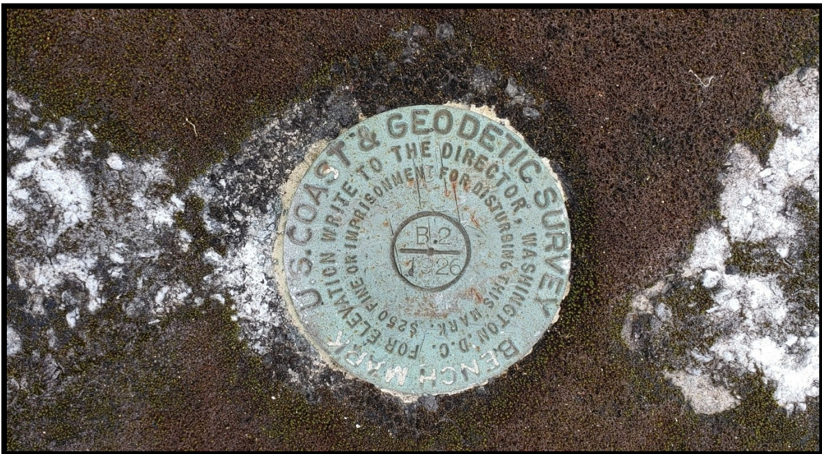
Figure 18. Close-up view of a 1926 U.S. Coast & Geodetic Survey Bench Mark located on the western wall of the bridge
