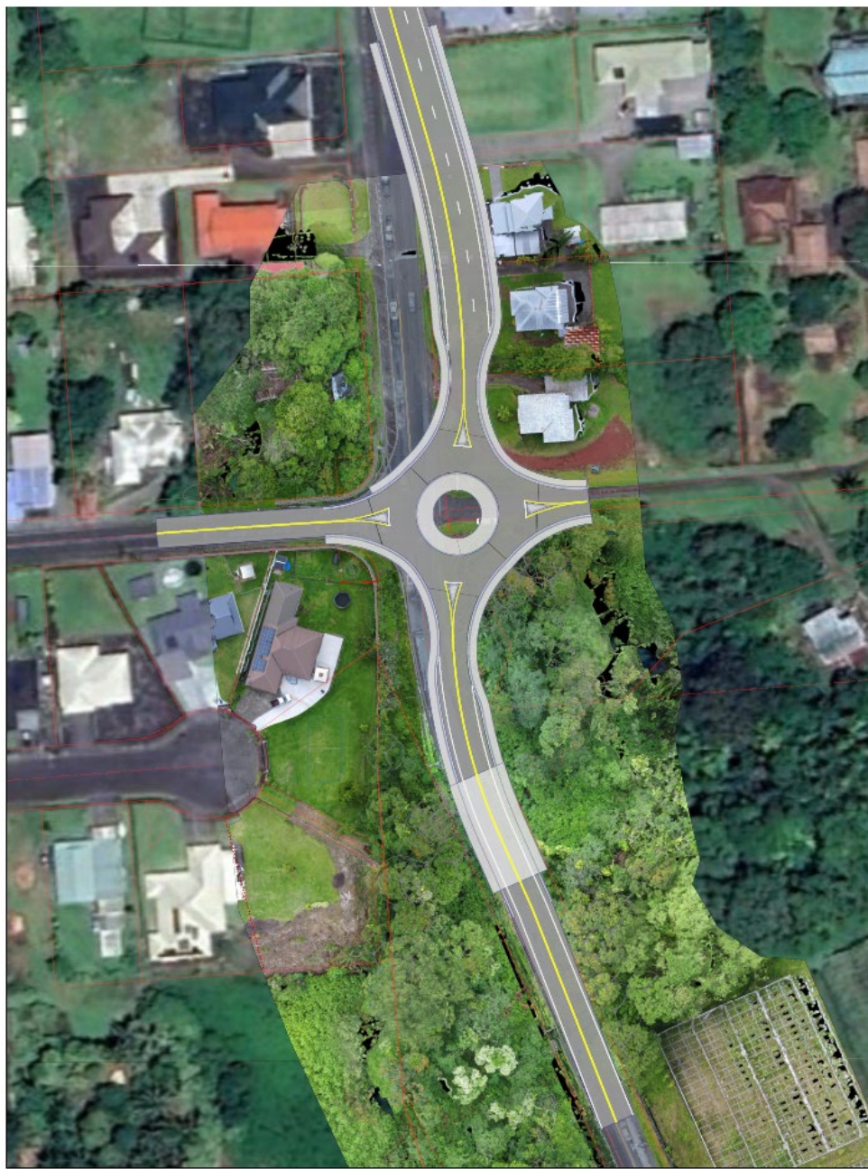
Figure 5: Schematic of Alternative B to the Proposed Action – New Roundabout at the Kilauea Avenue and Haihai Street Intersection
