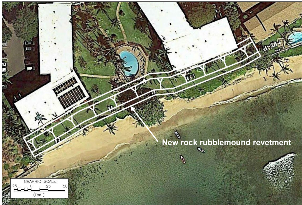
Figure 5-22 Conceptual plan view of a rock rubblemound revetment at KAN
