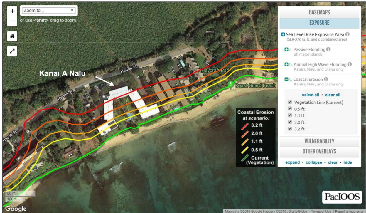
Figure 2. Screenshot of the Sea Engineering, Inc.’s Figure 2-4 from its Kanai A Nalu Beach Management & Erosion Plan from July 2019, showing coastal erosion with 0.5 to 3.2 feet of sea level rise.
