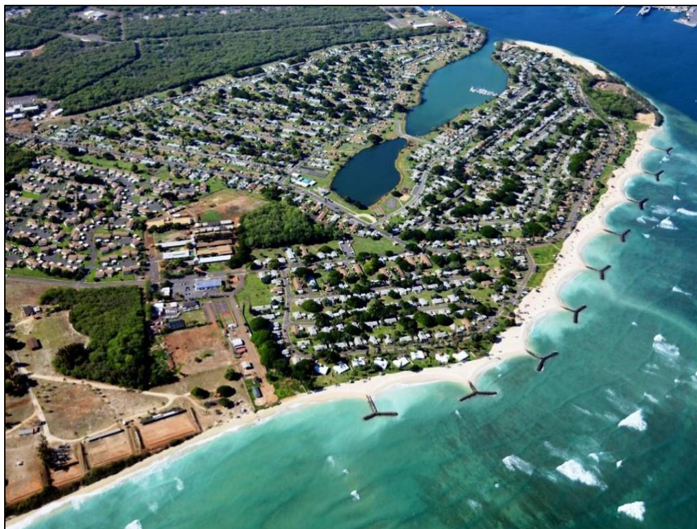
Figure 5-5 Beach restoration with T-head groins at Iroquois Point, Oahu (2017)
