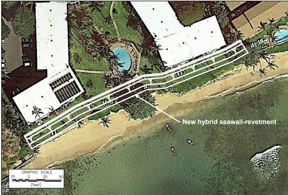
Figure 5-25 Conceptual plan view of a hybrid seawall-revetment at KAN
