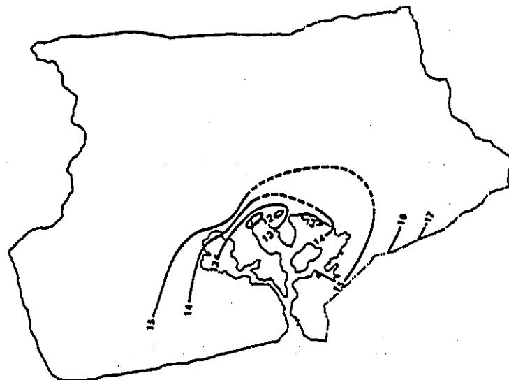
BASAL-WATER HEAD CONTOURS BASED ON MEASUREMENTS ON JANUARY 11, 1978.
