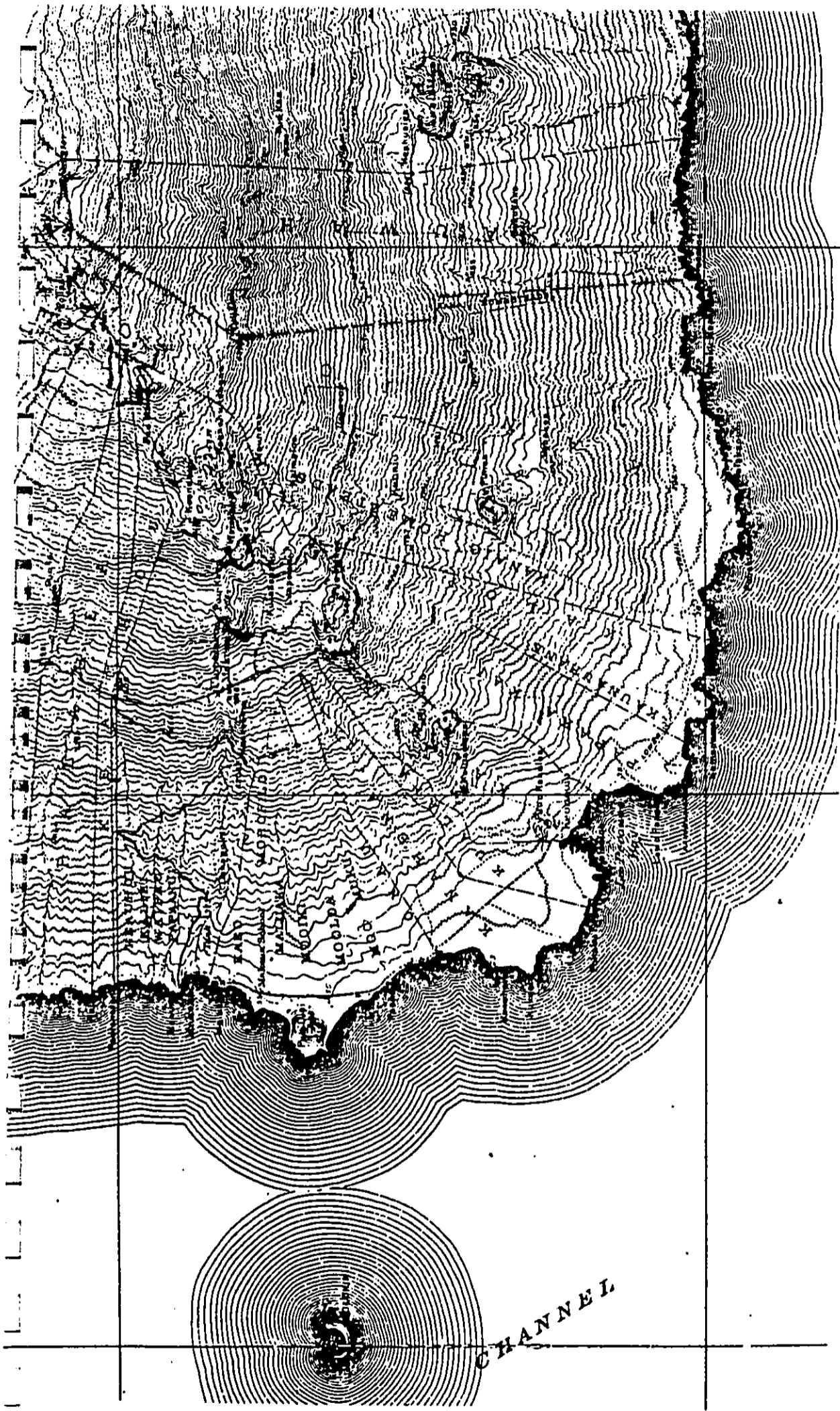
Fig. 23 . Portion of U.S.G.S. Mākena Quad. (1923-24), 1:62,500. Note lower trail along the coastline and Upper trail with its elevation varying between approximately 1600 to 2000 ft.
